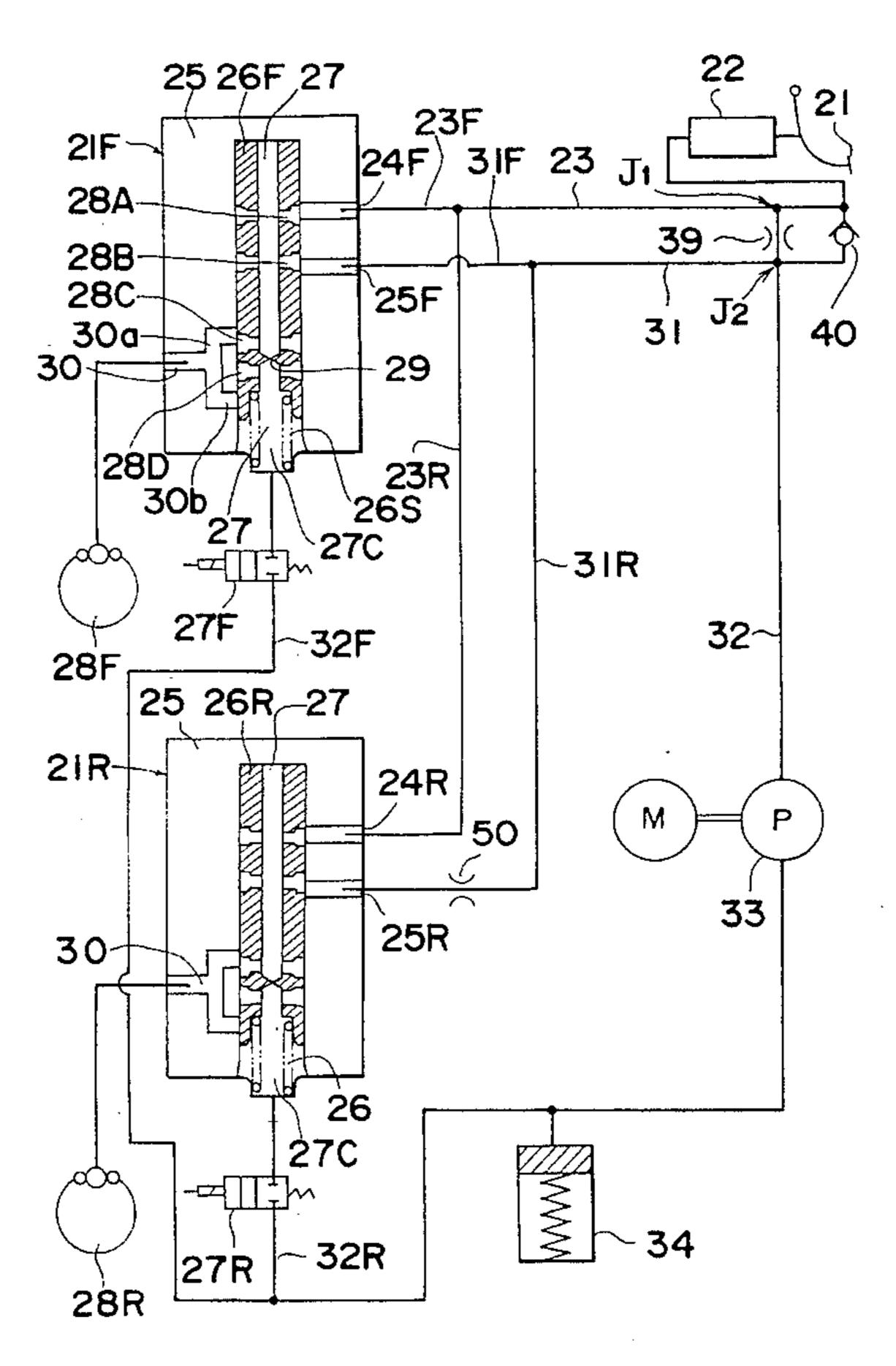
Fig. | Normal Braking Mode
