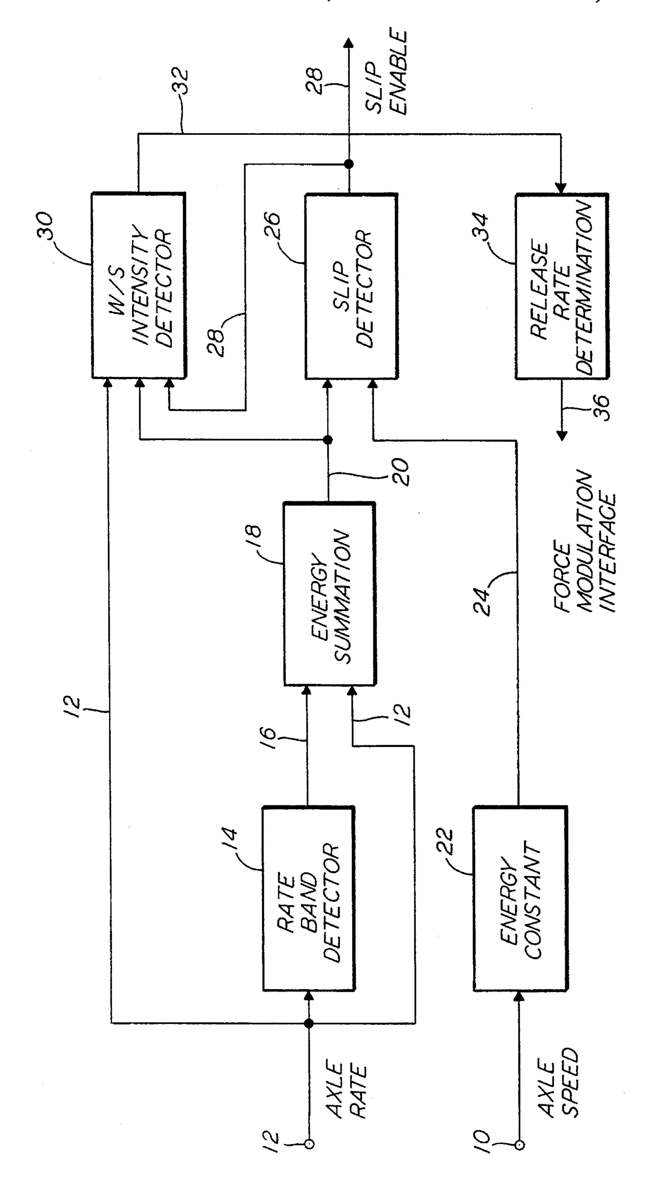
METHOD OF AND APPARATUS FOR THE COMBINED DETECTION OF SPEED VARYING ENERGY LEVEL WHEEL SLIP DETECTION AND DETERMINATION OF WHEEL SLIP INTENSITY OF A RAILWAY VEHICLE BRAKE SYSTEM
