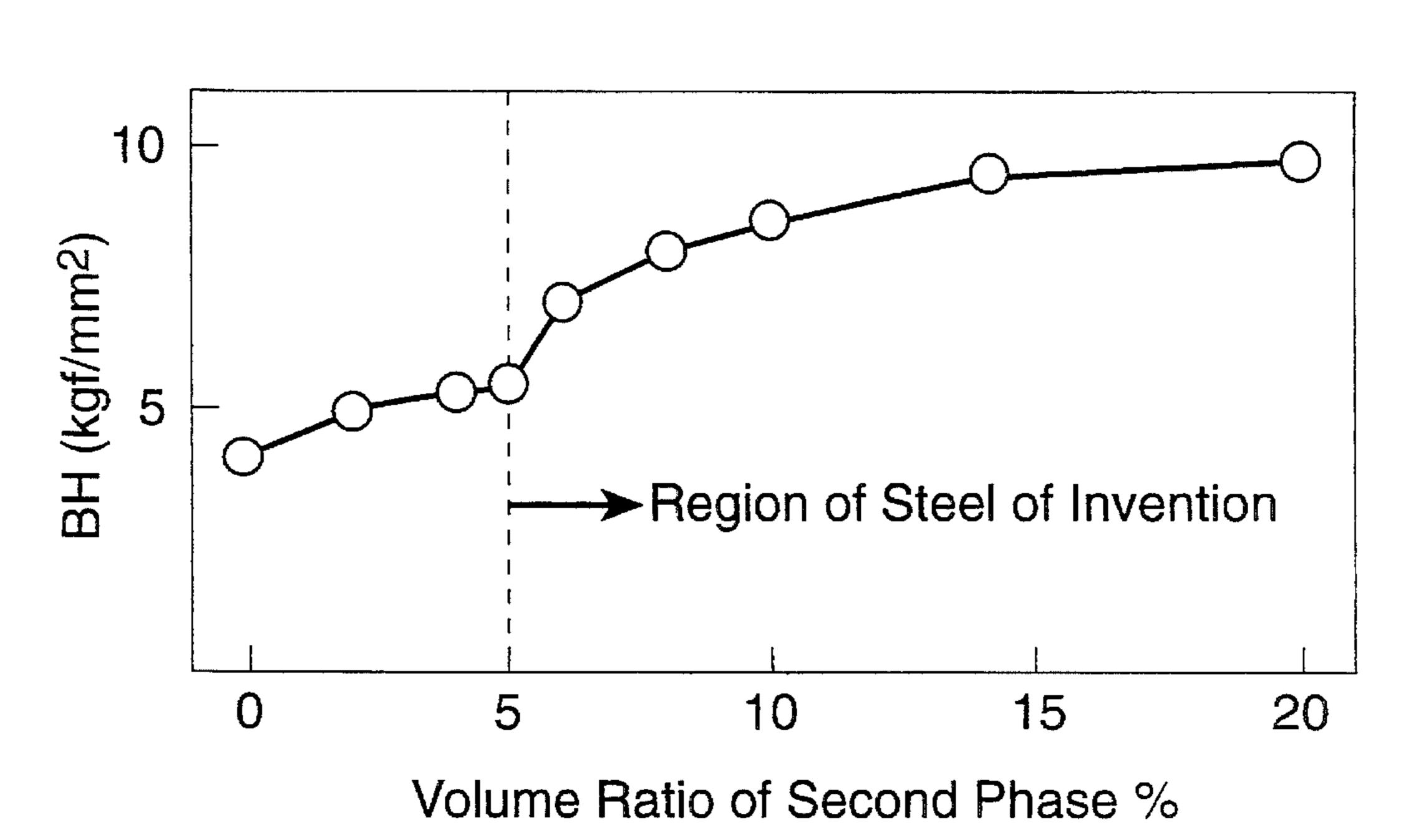
COLD ROLLED STEEL SHEET AND HOT DIP ZINC-COATED COLD ROLLED STEEL SHEET HAVING EXCELLENT BAKE HARDENABILITY, NON-AGING PROPERTIES AND FORMABILITY, AND PROCESS FOR PRODUCING SAME
