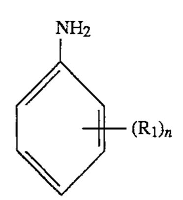
where  $R_1$  is  $C_1$ – $C_{10}$  alkyl or halogen and n is an integer from 0 to 3 are effective in increasing the motor octane number of aviation gasolines to 98 or greater without the presence of lead additives.
