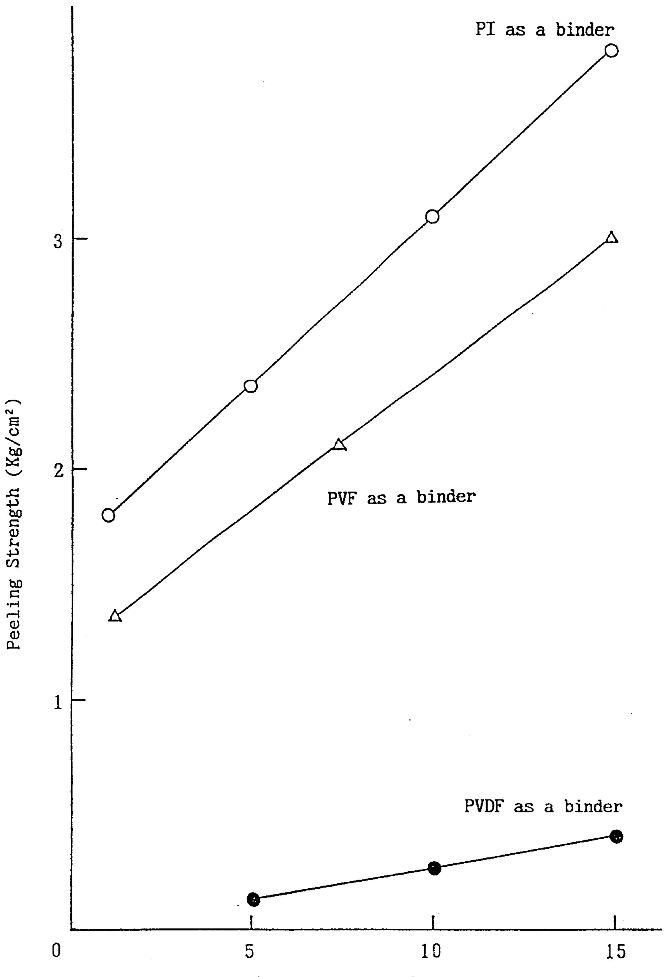
Mixing ratio (parts by weight) of each binder based on 100 parts by weight of graphite
