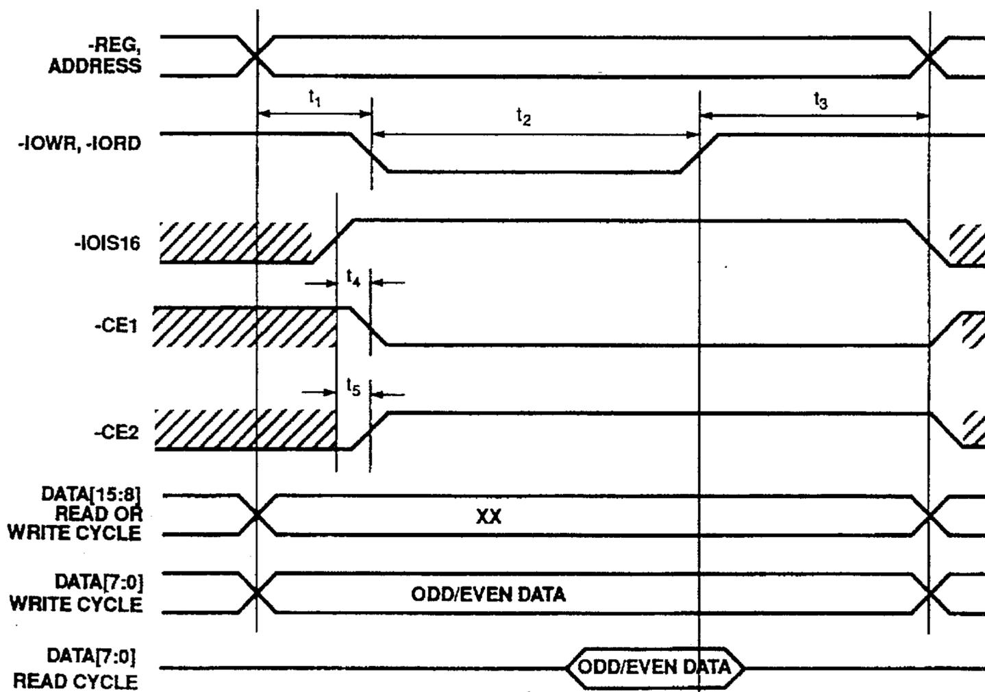
Figure 12–8. Word-To-Byte Conversion, Odd Byte I/O Read/Write Timing
