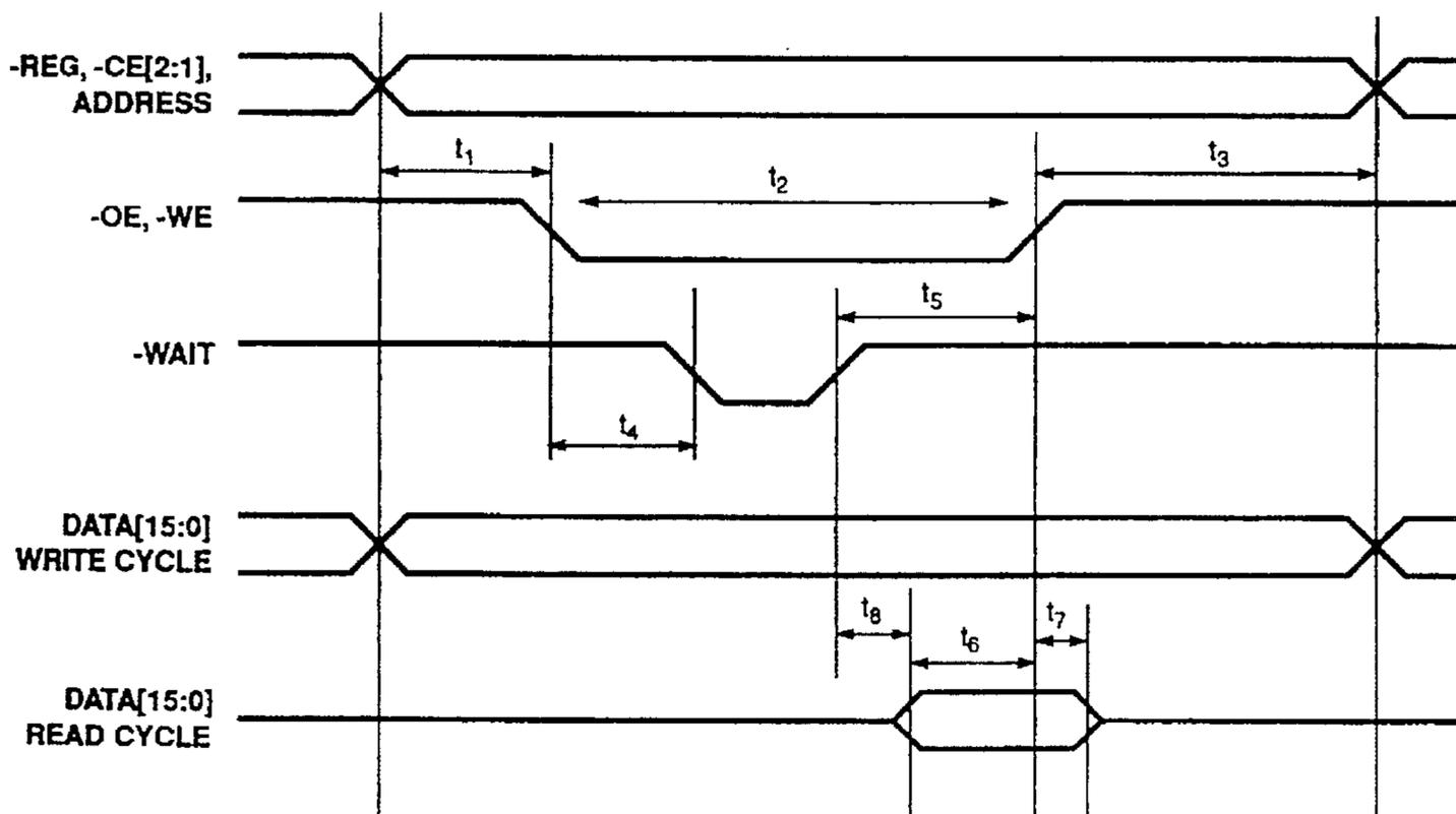
Figure 12–4. Memory Read/Write Timing
