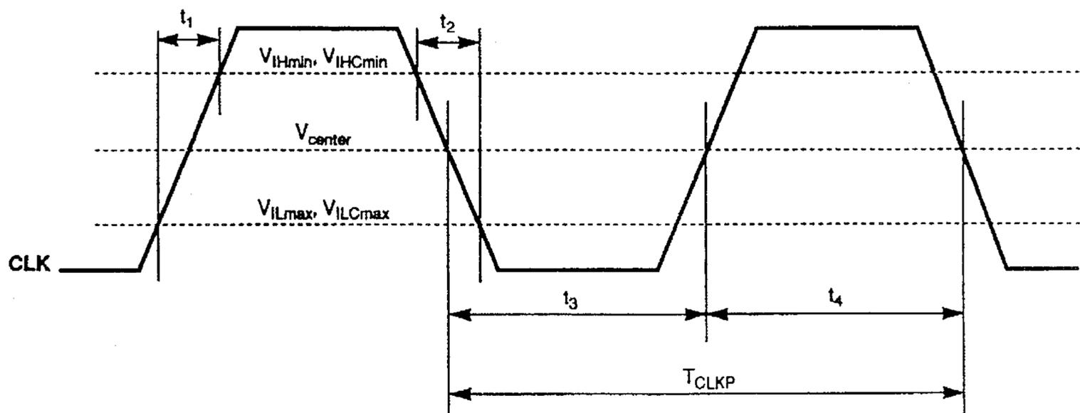
Figure 12-3. Input Clock Specification
