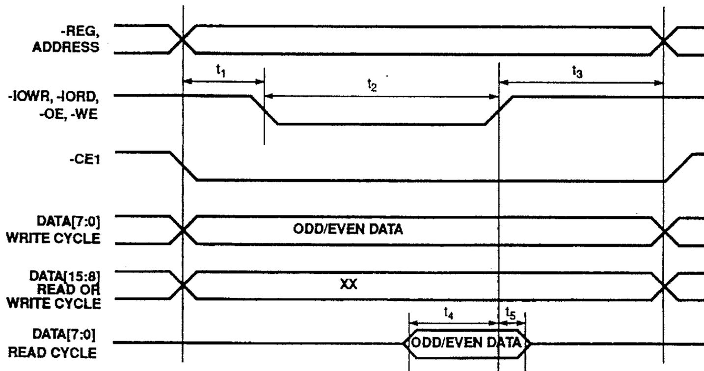
Figure 12-6. PCMCIA Read/Write Timing When Host Is 8-Bit (SBHE Tied High)
