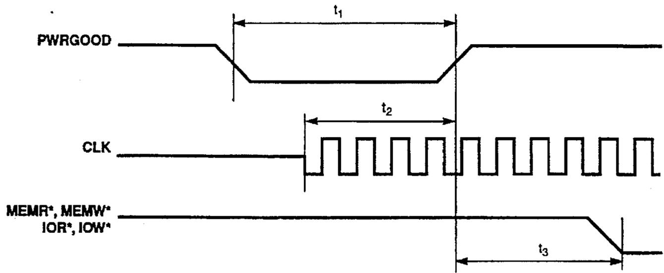
Figure 12–2. Reset Timing
