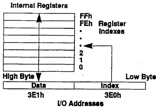
Figure 3-1. Indexed 8-Bit Register Structure
