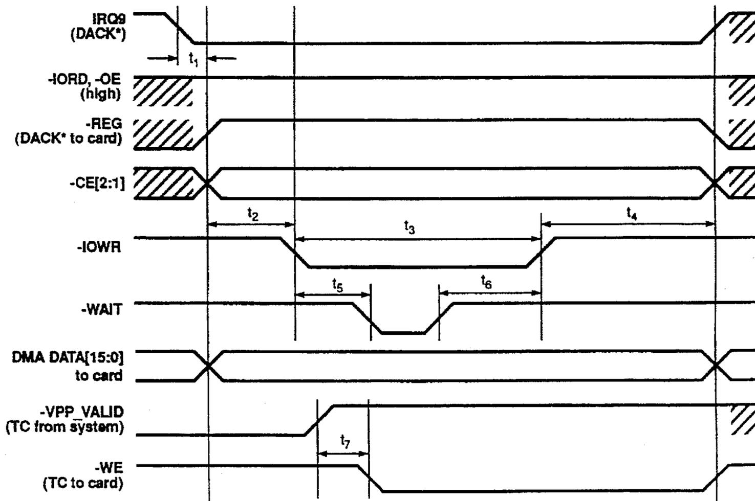
Figure 12-9. DMA Read Cycle Timing
