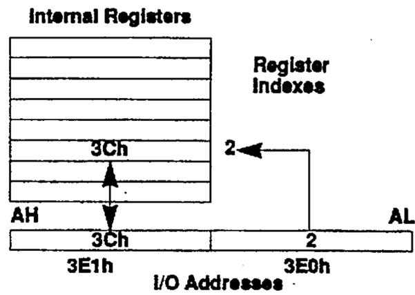
Figure 3-2. Indexed 8-Bit Register Example
