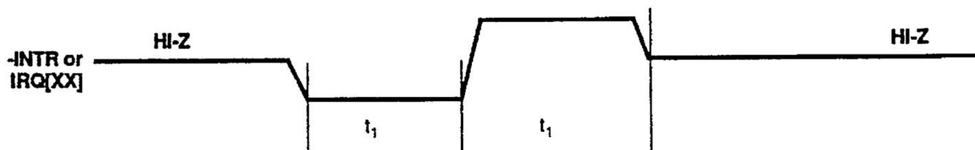
Figure 8-1. Pulse Mode Interrupts
