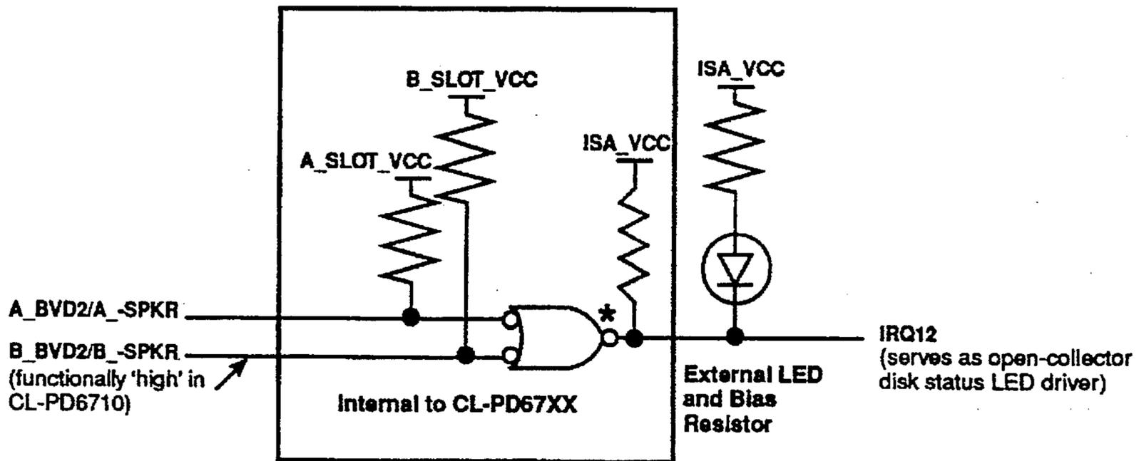
Figure 10-1. Disk-Status LED Logic for ATA Mode
