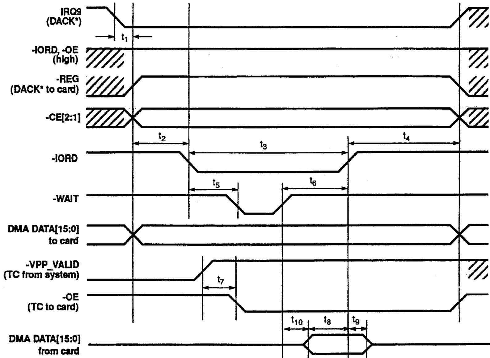
Figure 12-10. DMA Write Cycle Timing
