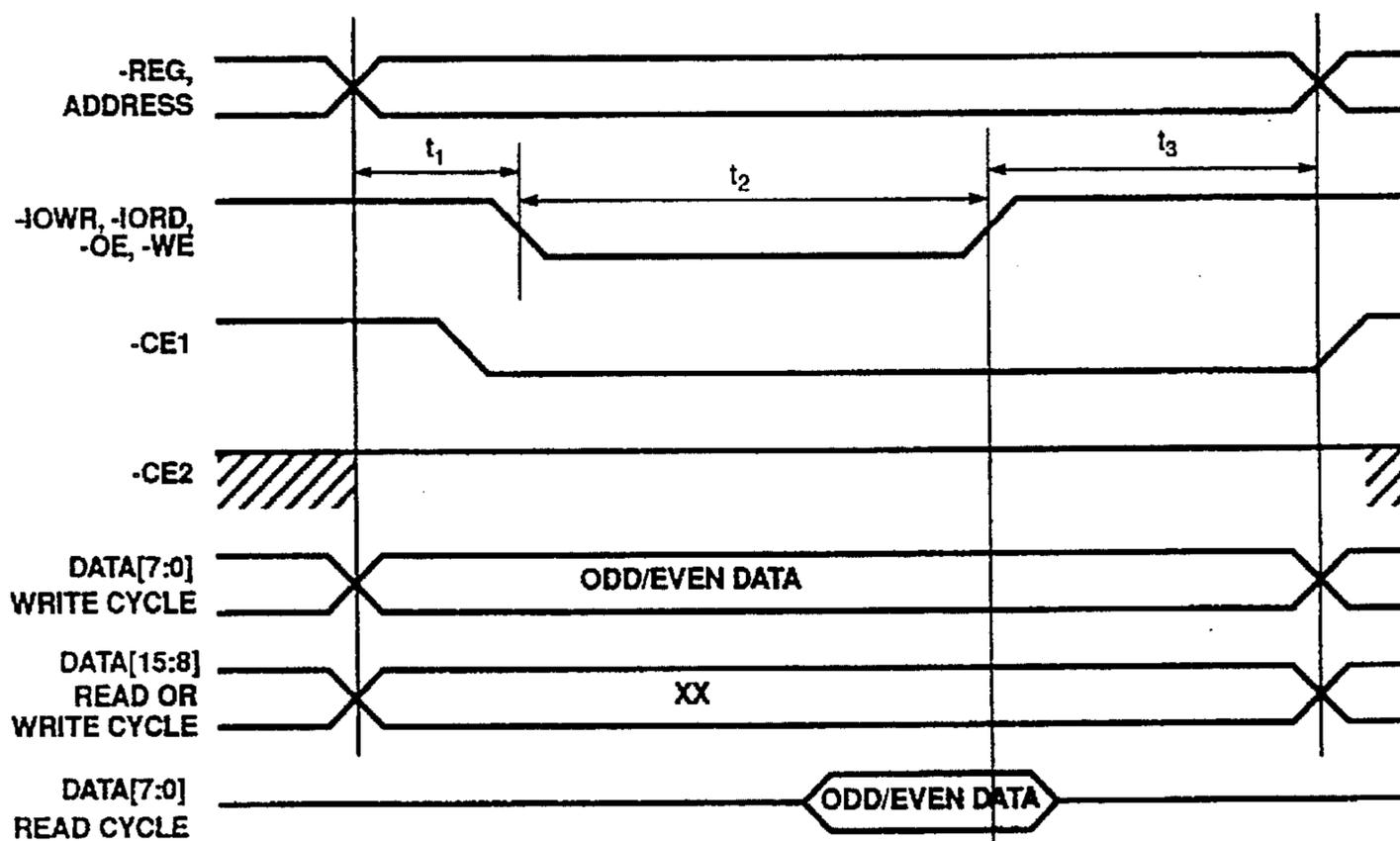
Figure 12-7. Normal Byte Read/Write Timing (e.g., All Other Byte Accesses, Including Odd I/O Cycles Where -IOIS16 Is Low)
