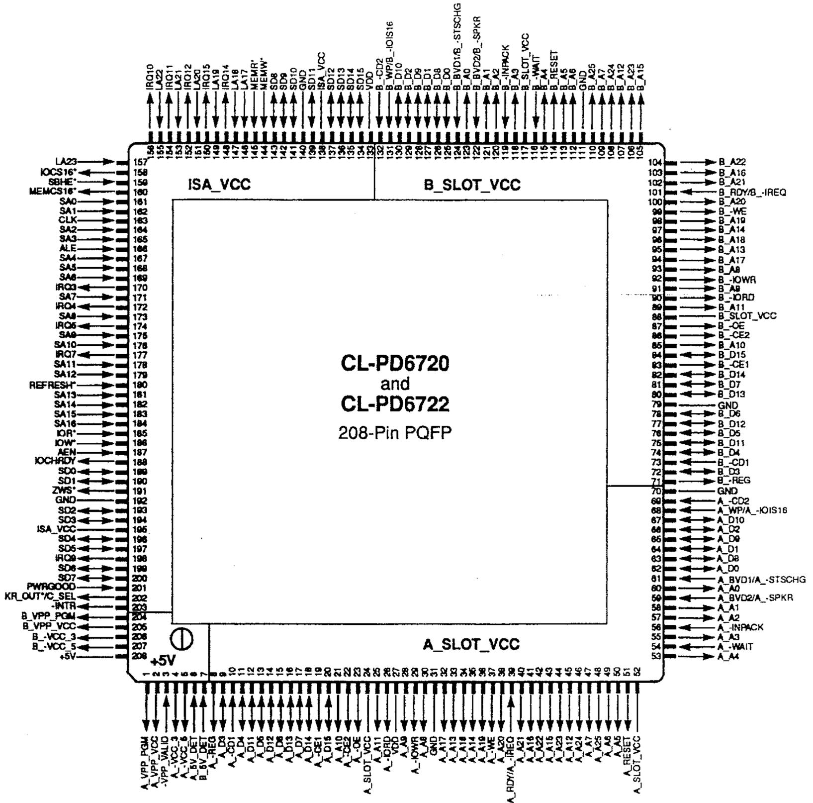
Figure 2-2. CL-PD672X Pin Diagram (top view, with pin names)
