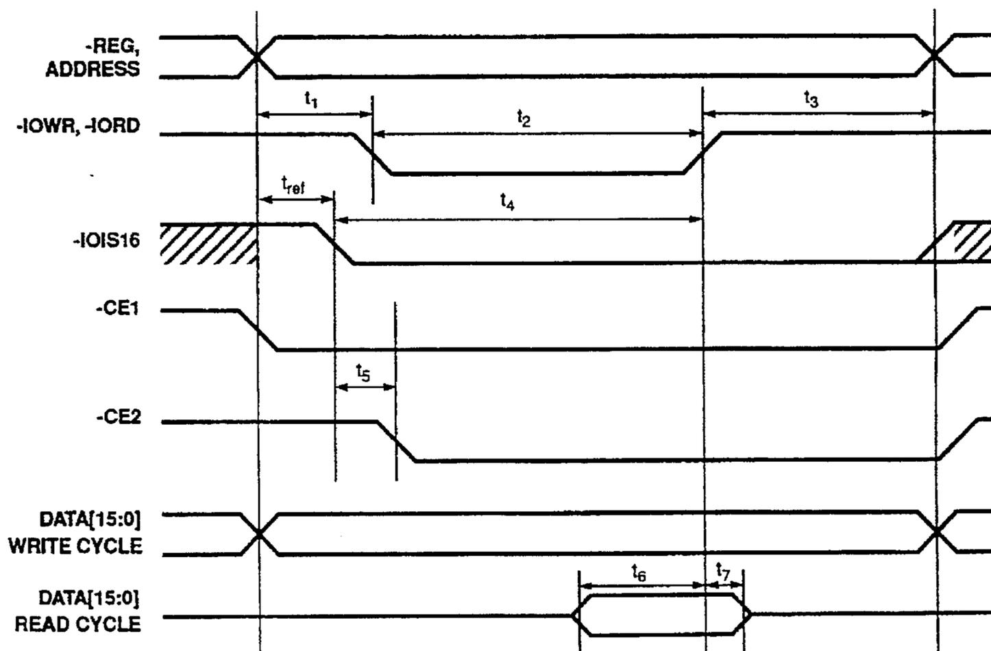
Figure 12–5. Word I/O Read/Write Timing
