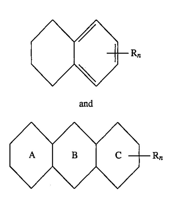
where one of the rings A, B or C has a benzene structure, R is alkyl of from 1 to 10 carbon atoms and n is an integer from 1 to 6. The remainder of the aromatics fraction are monoand di-aromatics which comprise one and two ring aromatics bearing at least one alkyl substituent typified by R as defined above. Another important feature is that the benzene, naphthalene and methyl substituted benzenes and naphthalenes concentrations are each less than 100 wppm.
