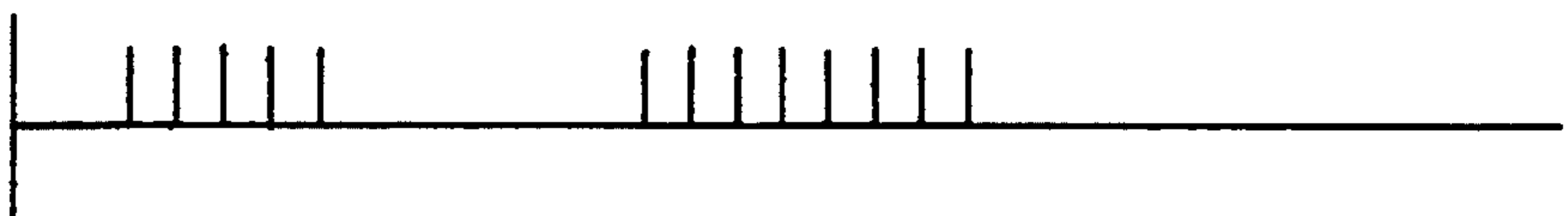
FIG. 7C TRANSIENT EDGE DETECTION SIGNAL
