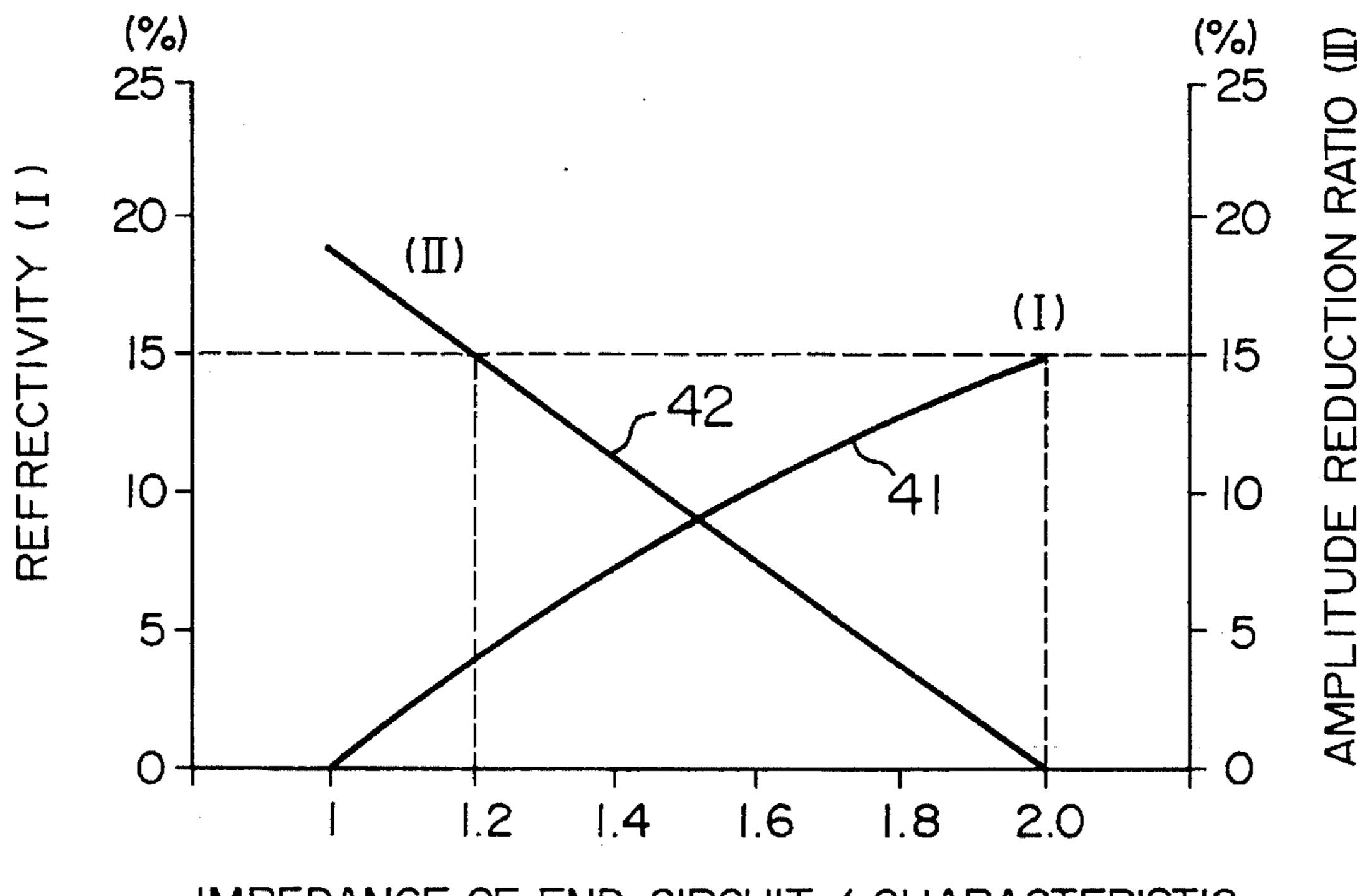
IMPEDANCE OF END CIRCUIT / CHARACTERISTIC IMPEDANCE OF TRANSMISSION PATH
