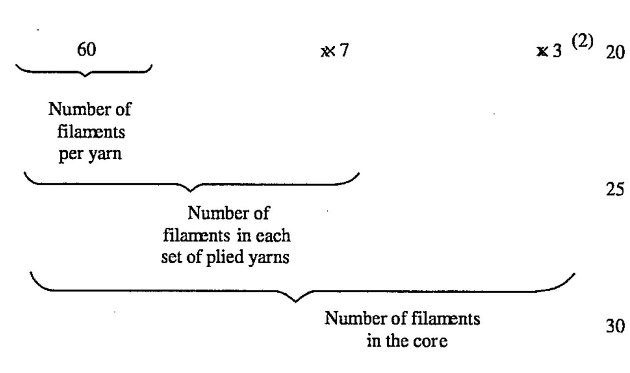
It will be understood that in the foregoing example, three sets of plied yarns are back twisted to form the core, with each front twisted plied yarn consisting of seven 60 filament yarns.
