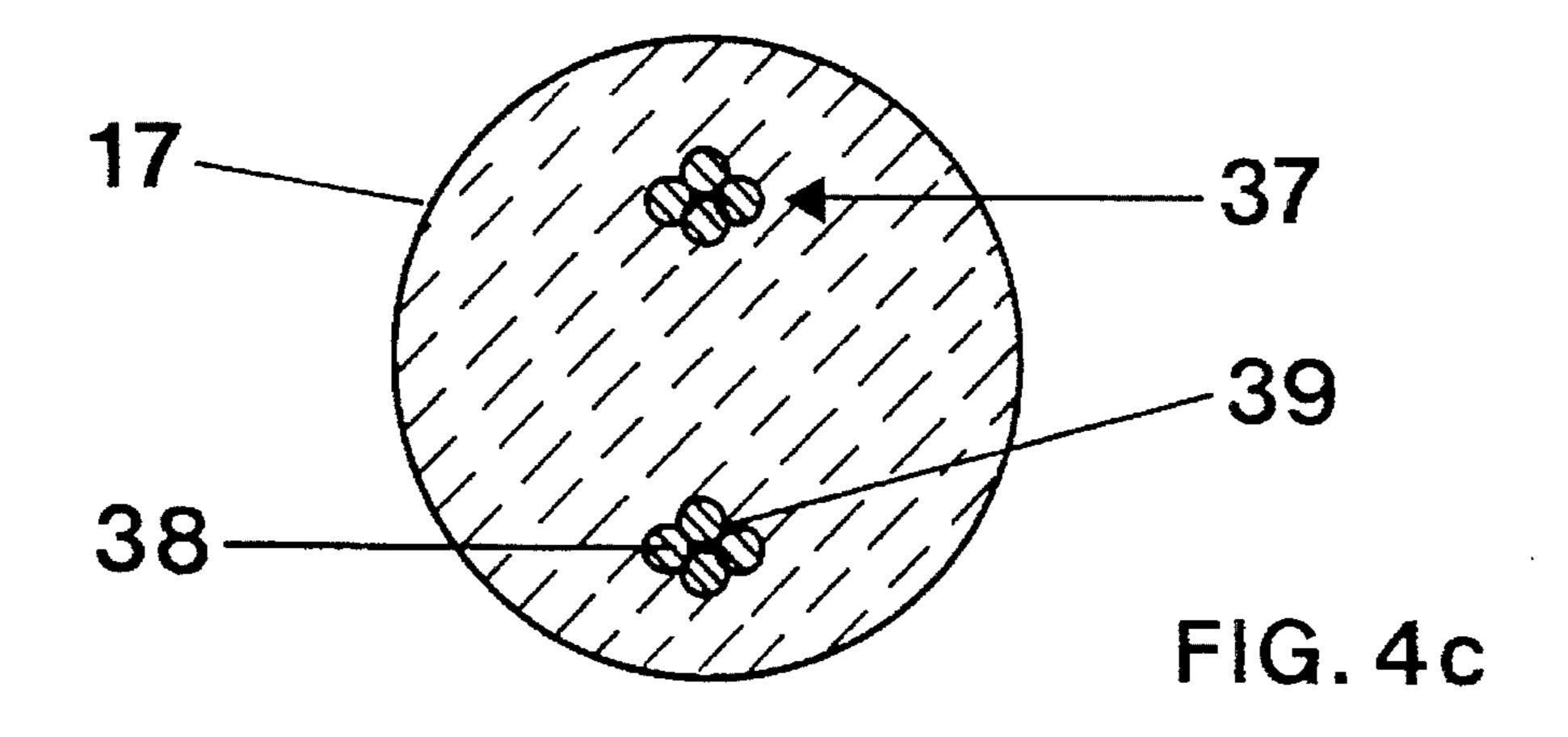
HIGH-PRESSURE DISCHARGE LAMP WITH CERAMIC DISCHARGE VESSEL AND CERAMIC SEALING MEANS HAVING LEAD-THROUGH COMPRISING THIN WIRES HAVING A THERMAL COEFFICIENT OF EXPANSION SUBSTANTIALLY LESS THAN THAT OF THE CERAMIC SEALING MEANS
