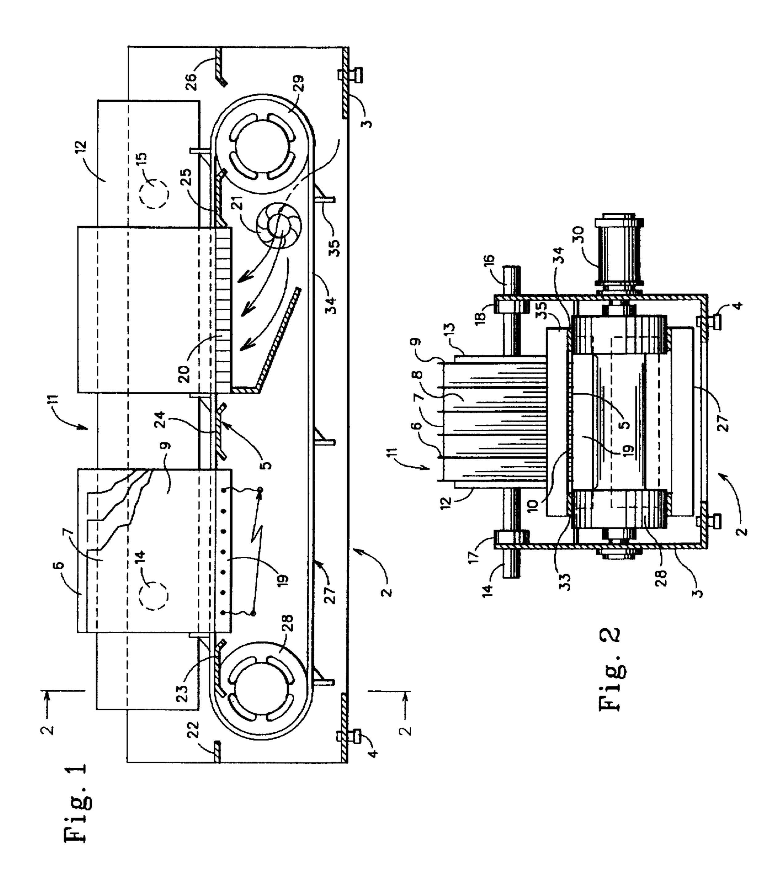
a thermoplastic adhesive to form a volume and comprising 5 a frame with two mutually and adjustably spaced supports acting as an insertion shaft for the covers, said shaft being fitted at its lower side with a heater, and further comprising
