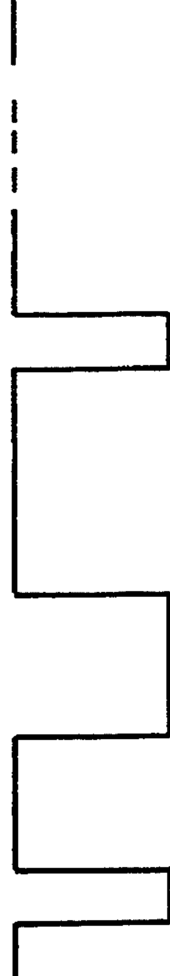
OUTPUT SIGNAL FROM COMPARATOR 48 (PULSE SIGNAL)
