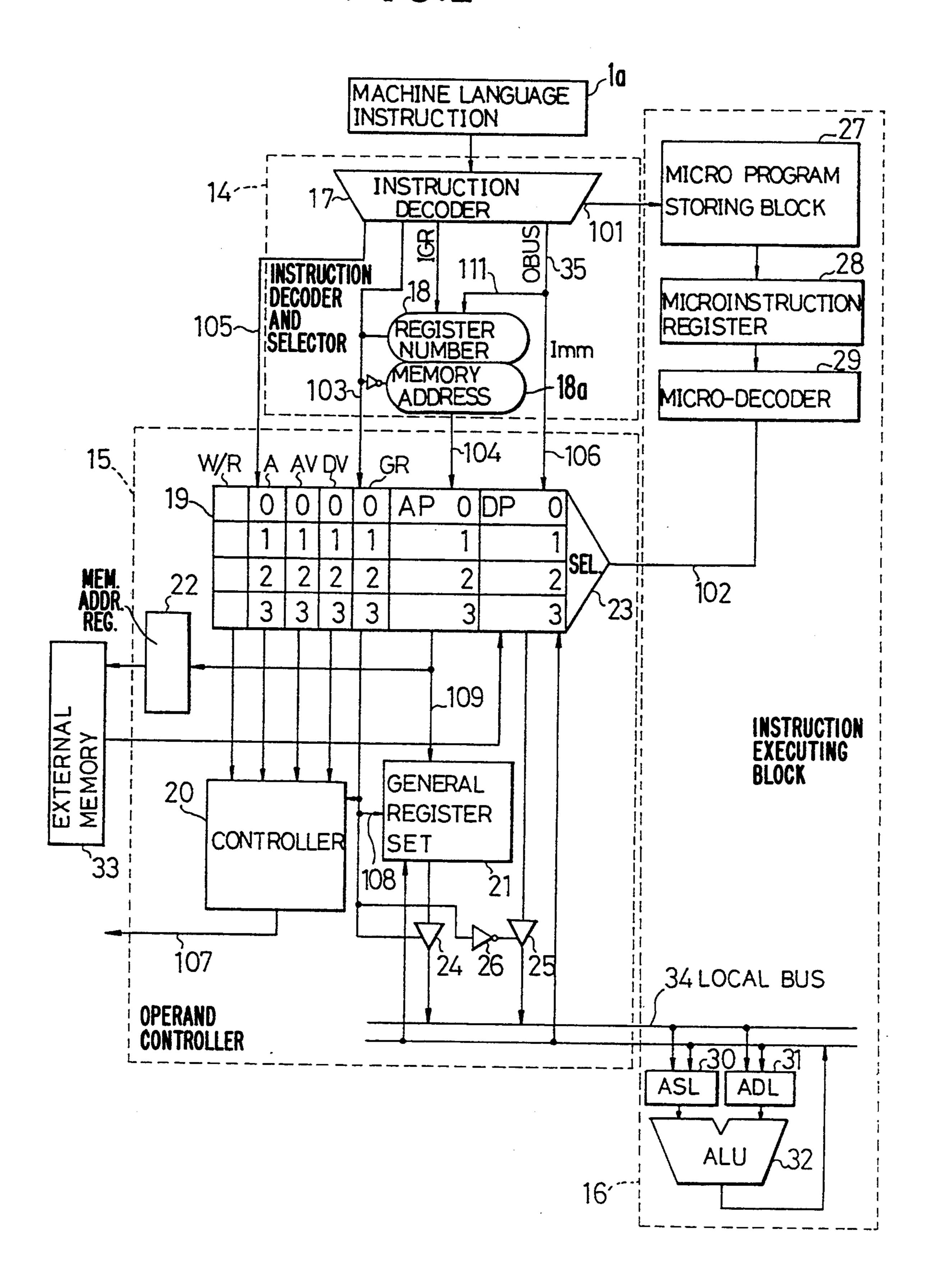
PROCESSOR HAVING DIFFERENT OPERAND SOURCE INFORMATION TEMPORARILY STORED IN PLURAL HOLDING REGISTERS TO AVOID USING MICROPROGRAM ROM CAPACITY FOR SUCH INFORMATION
