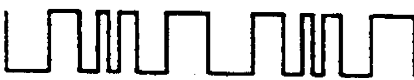
OUTPUT SIGNAL AT OUTPUT TERMINAL
