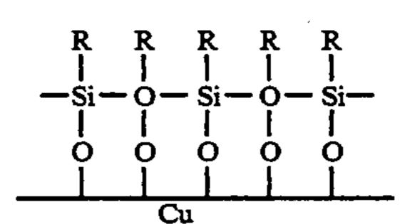
wherein R is an organic functional group such as vinyl group, glycidoxy group, amino group, and mercapto group, etc. Thus coated clad laminate is dried in such a manner as a natural drying, a heat drying, or a vacuum drying, to obtain the internal composite layer. For example, the coated clad laminate is dried under the atmospheric pressure at a temperature of 80° C. to 150° C.
