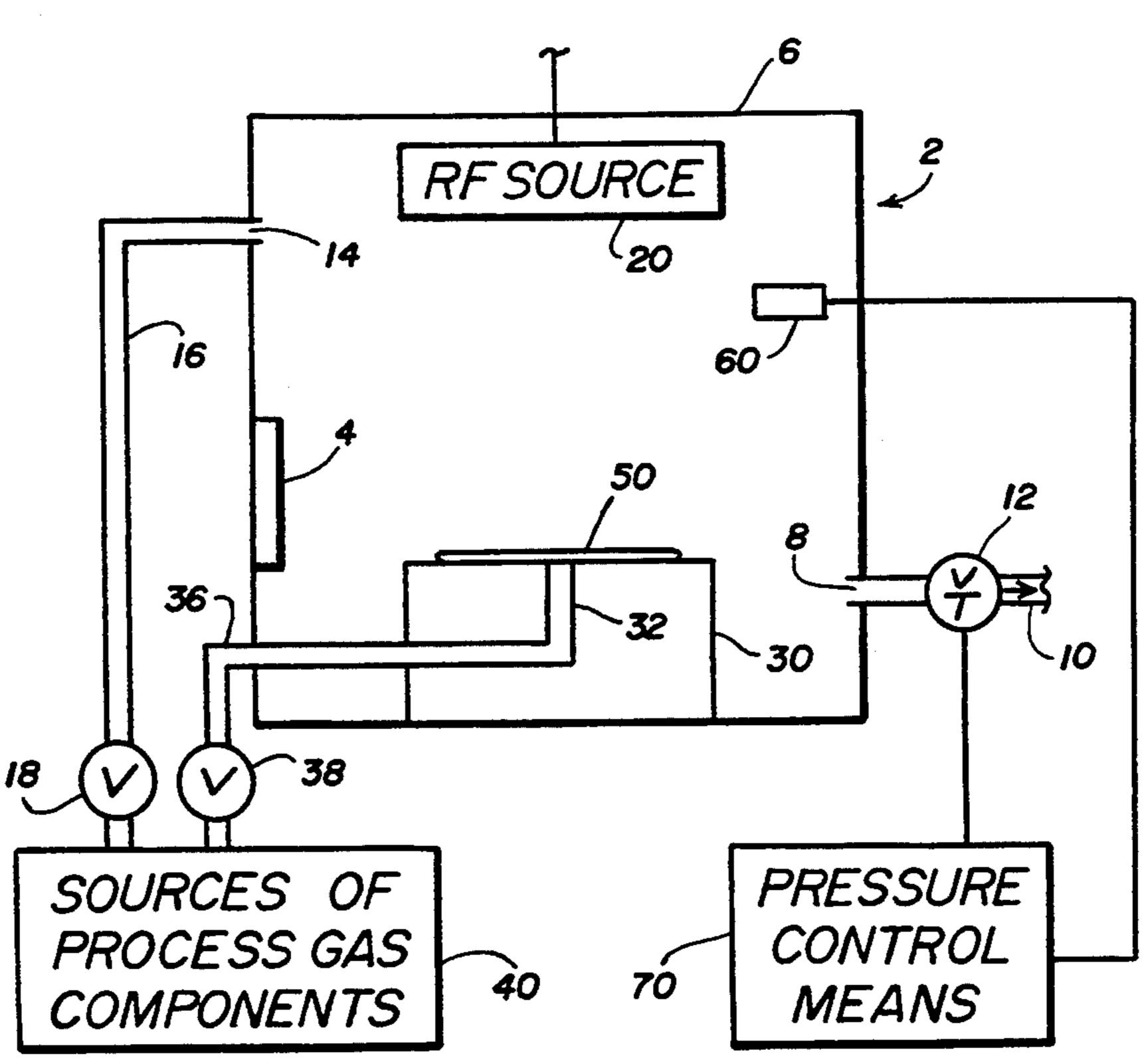
NONSEALINGLY SUPPORTING A SEMICONDUCTOR WAFER ON A HEATSINK IN A PLASMA ETCHING CHAMBER
