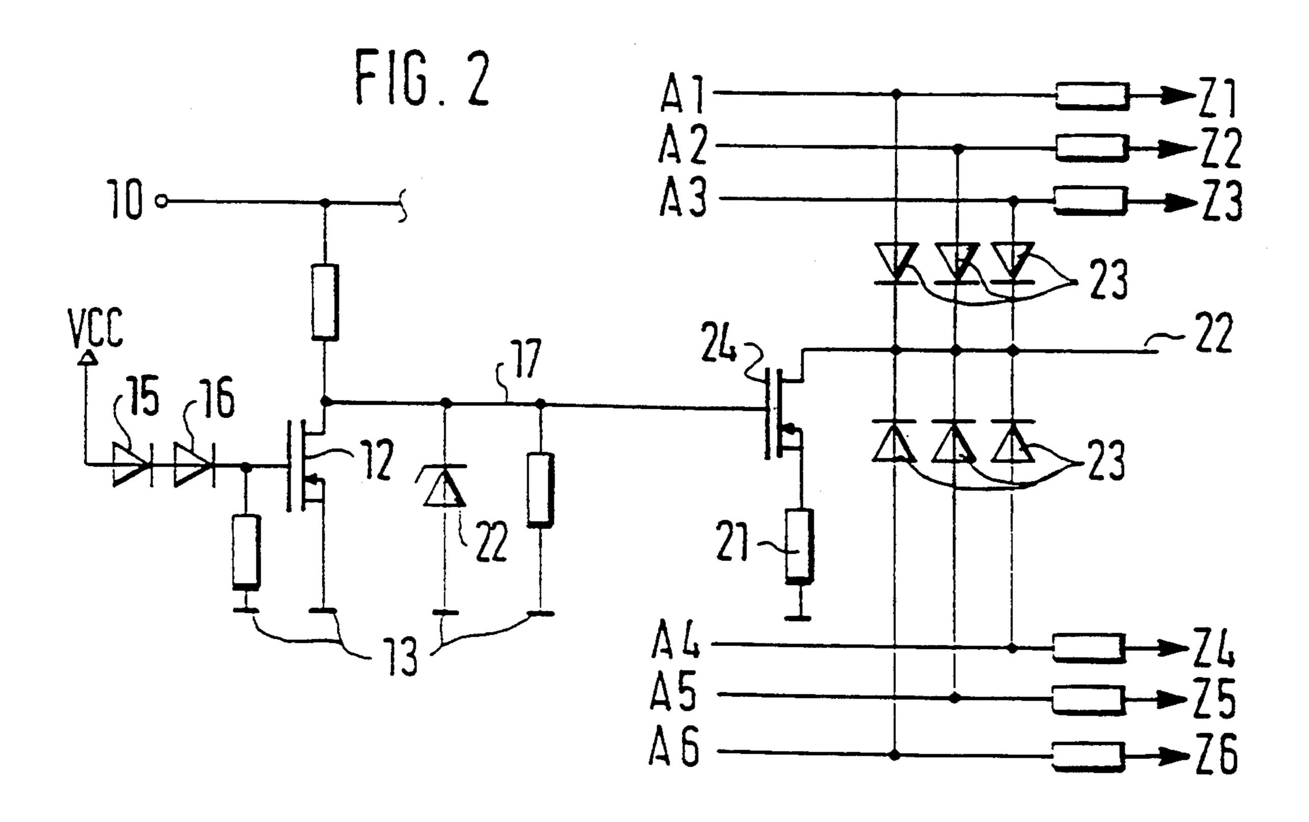
FIG. 2 shows a second embodiment of an ignition system in accordance with the present invention.
