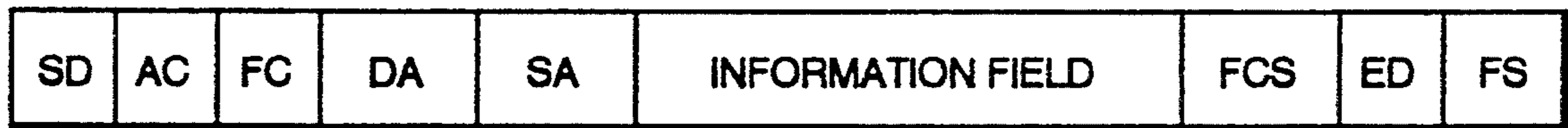
FIG. 4D FRAME STRUCTURE (IEEE 802.5)
