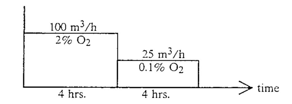
In the first period, customer requires a flow of 100 m<sup>3</sup>/h inert at a maximum O<sub>2</sub> content of 2%. In a second period, flow need falls down to 25 m<sup>3</sup>/h at a purity of 0.1% O<sub>2</sub> max.
