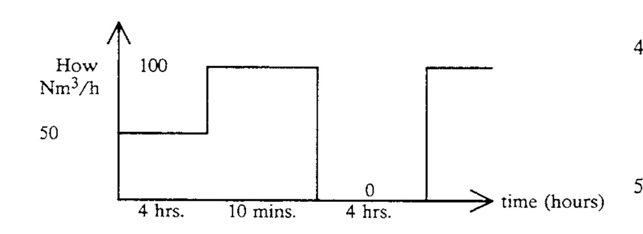
Basic flow is 50 Nm<sup>3</sup>/h at 2% O<sub>2</sub> content. Surges of 100 Nm<sup>3</sup>/h consumption at 2% O<sub>2</sub> occur during 10 mins every 4 hrs.
