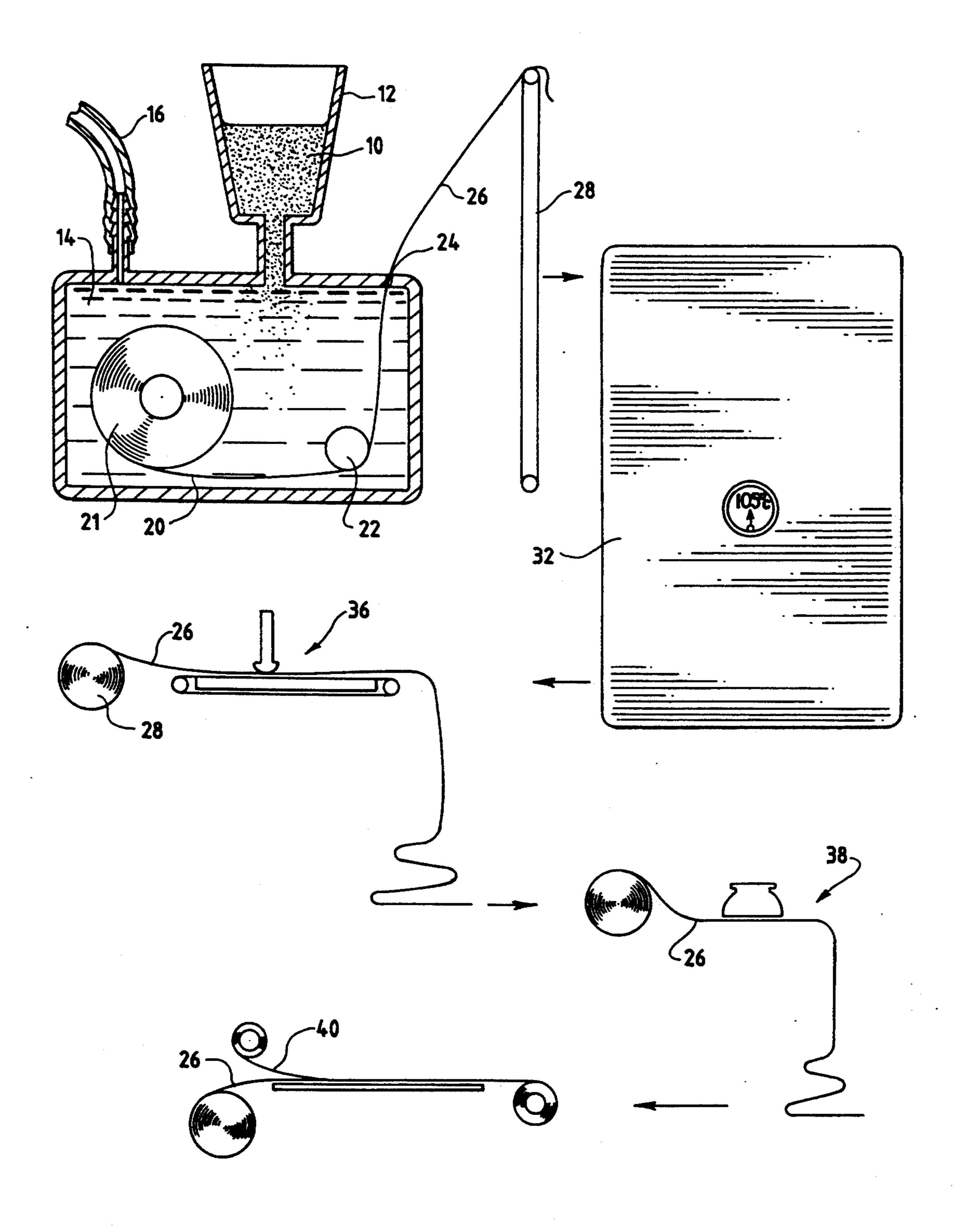
LOW ABRAISION MATERIAL COMPRISING A FIBROUS MATRIX IMPREGNATED WITH A POLYURETHANE RESIN WHEREIN FIBER ENDS ARE EXPOSED ON AT LEAST ONE SURFACE OF THE MATERIAL
