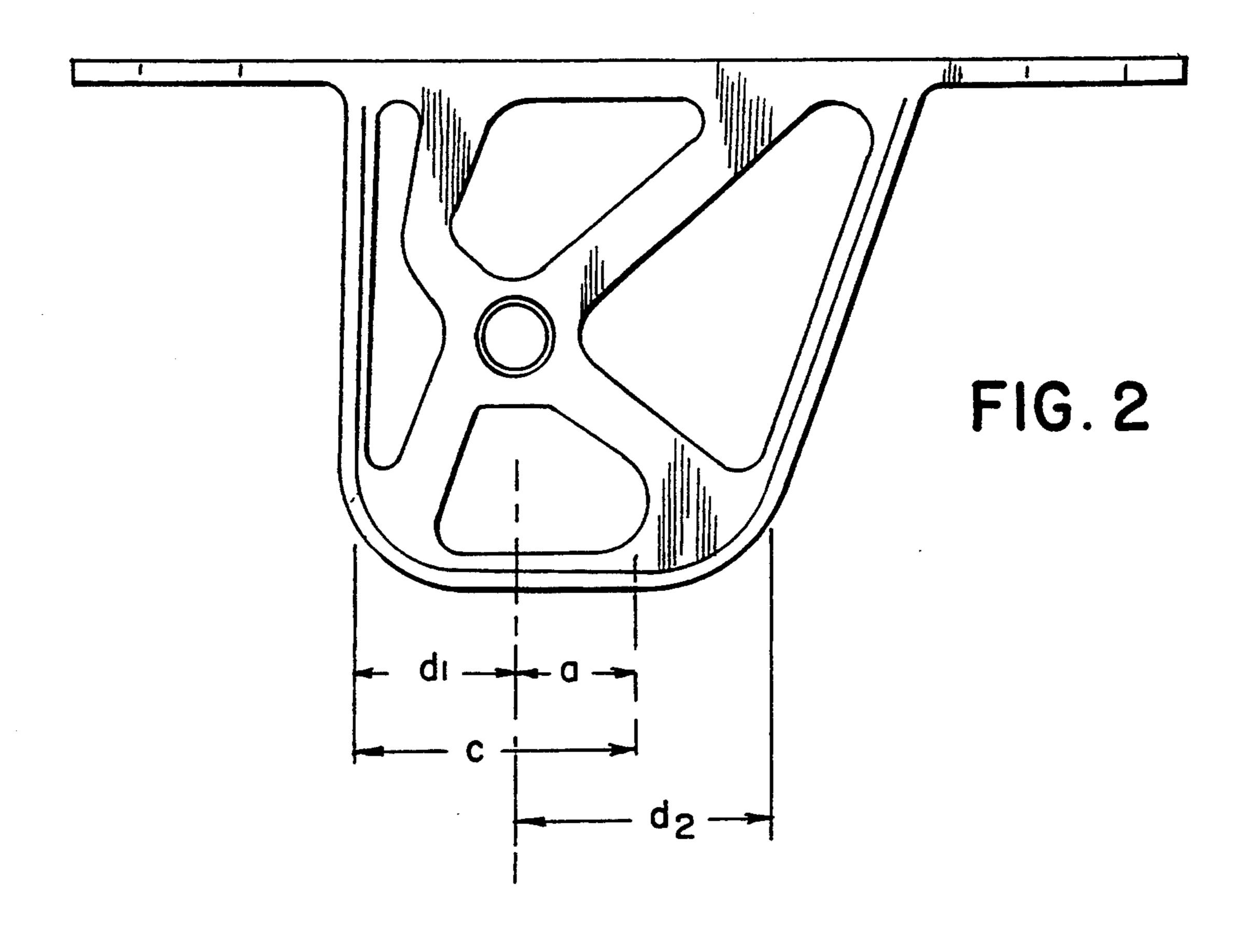
ELASTIC SUSPENSION FOR ATTACHING DYNAMICALLY STRESSED FUNCTION PARTS
