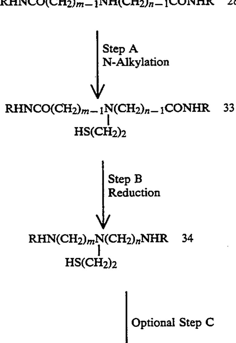
In Scheme VIII, step A the appropriately substituted diamide (28) prepared in Scheme VI, step D is mono-N-alkylated with ethylene sulfide to provide the appropriately substituted mono-N-alkylated diamide described by structure (33).
