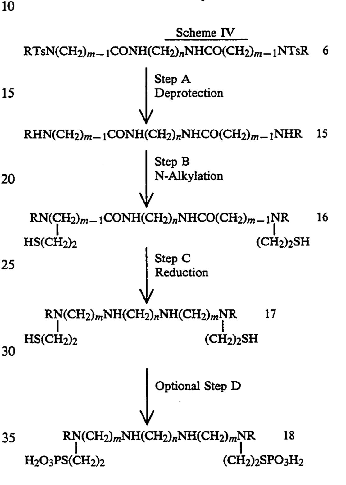
In Scheme IV, step A the diamide (6) prepared in Scheme II, step A is deprotected under conditions well known in the art to provide the deprotected diamide described by structure (15).
