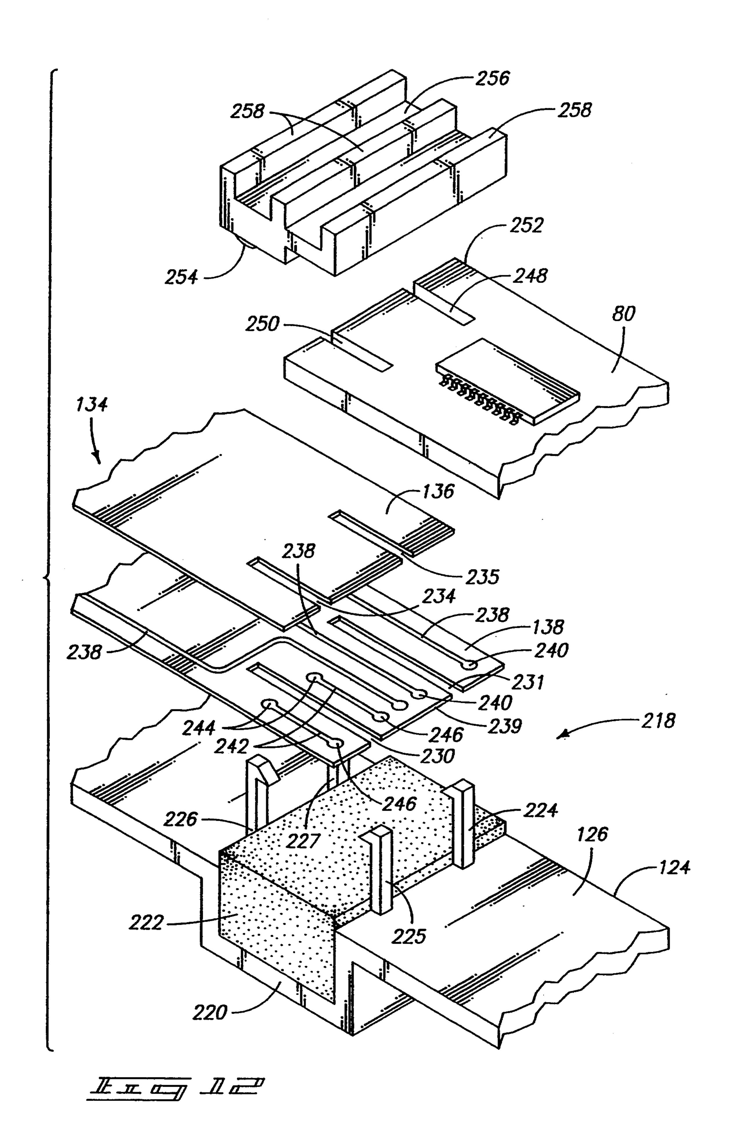
COMPUTER KEYBOARD WITH INTEGRAL DOME SHEET AND SUPPORT PEGS
