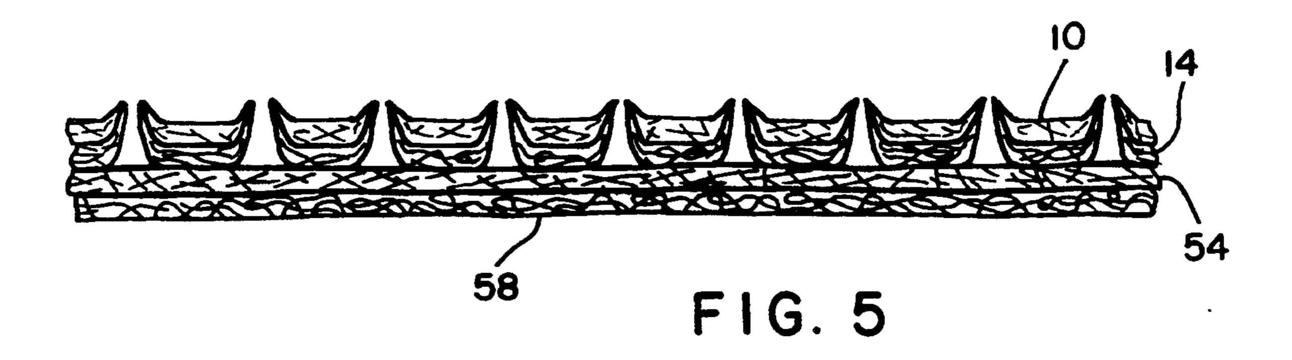
APERTURED ABRASIVE ABSORBENT COMPOSITE NONWOVEN WEB
