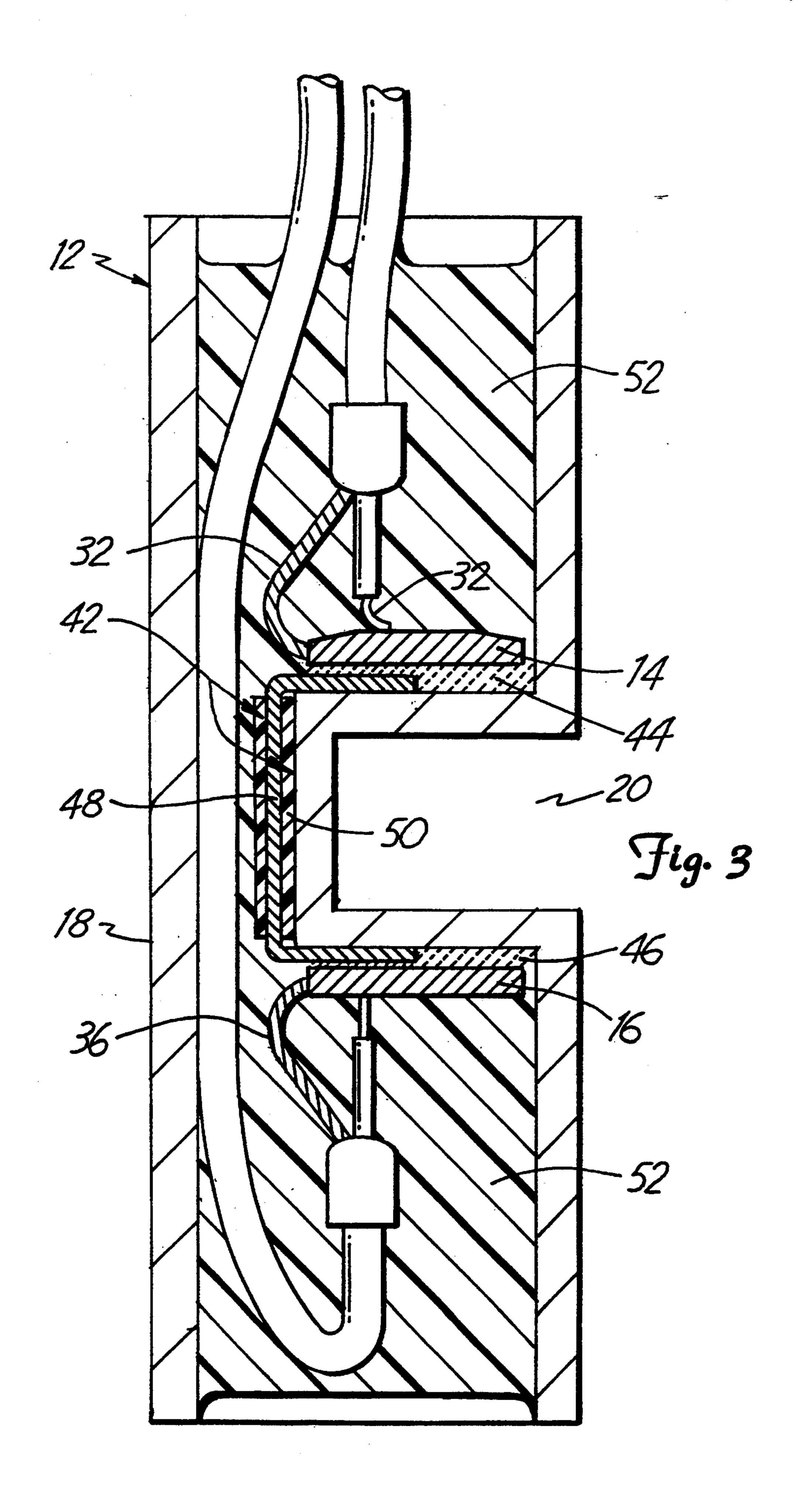
FIG. 3 is a detailed cross sectional view of support structure for an ultrasonic liquid level sensor in accor-
