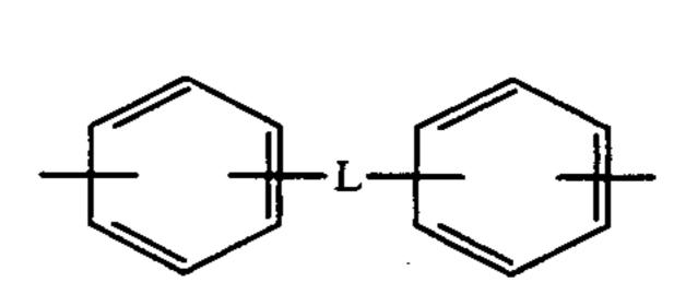
wherein L is a direct bond, alkylene of 1-6 carbon atoms, alkylidene of 2-6 carbon atoms or SO<sub>2</sub>. These represent, for example bisphenols F, A and S, catechol, resorcinol, 0,0'-biphenol and p,p'-biphenol. The various phenols may be substituted on the respective phenyl ring by such non-reactive substitutes such as hologen, alkyl and the like.
