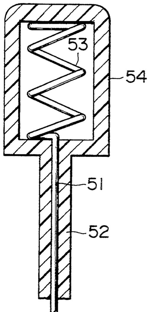
**RETRACTABLE ANTENNA DEVICE HAVING A
