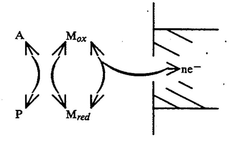
where A=analyte; P=product; and  $M_{ox}$  and  $M_{red}$  are the oxidized and the reduced forms of the mediator, respectively.
