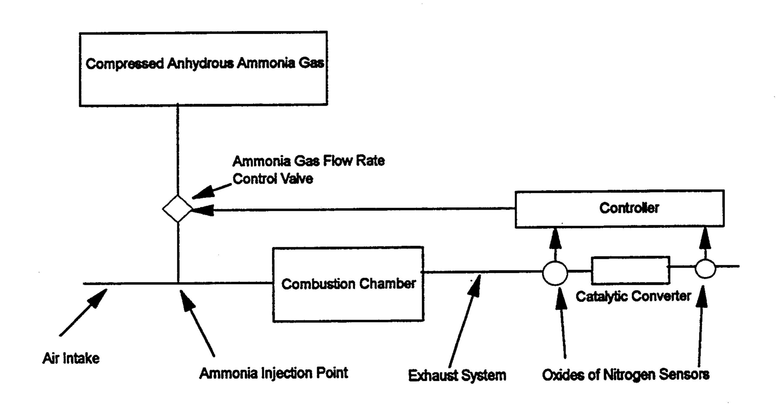
A System For Reducing Oxides Of Nitrogen
