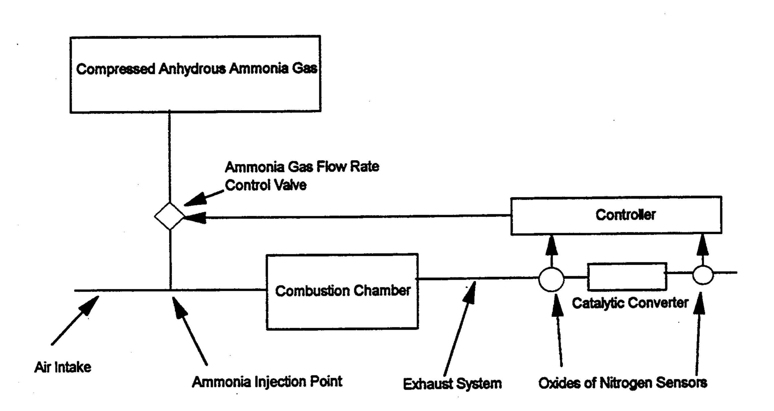
A System For Reducing Oxides Of Nitrogen
