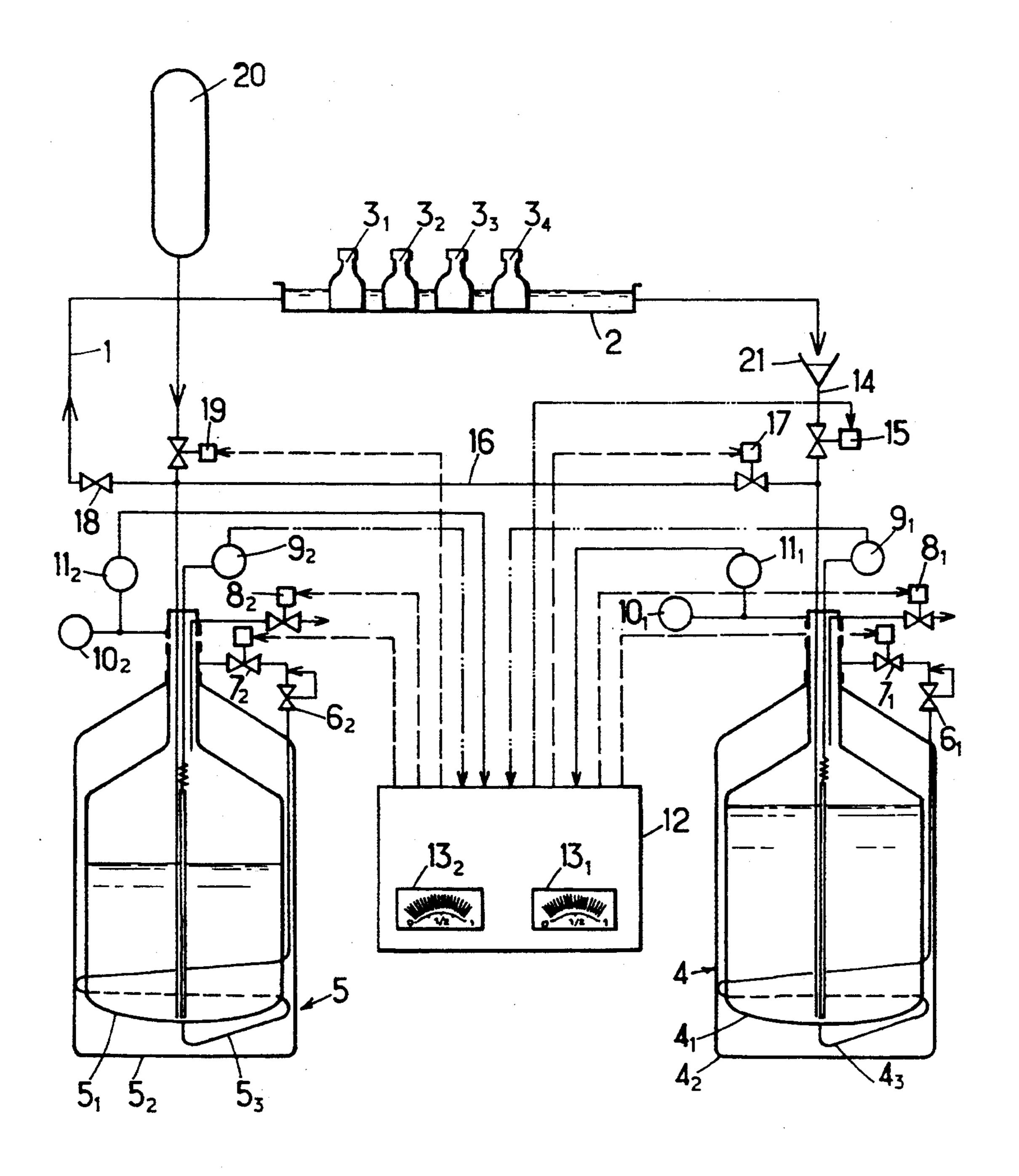
DEVICE FOR RECYCLING A CRYOGENIC LIQUID AND ITS USE IN AN APPARATUS FOR FREEZING PRODUCTS
