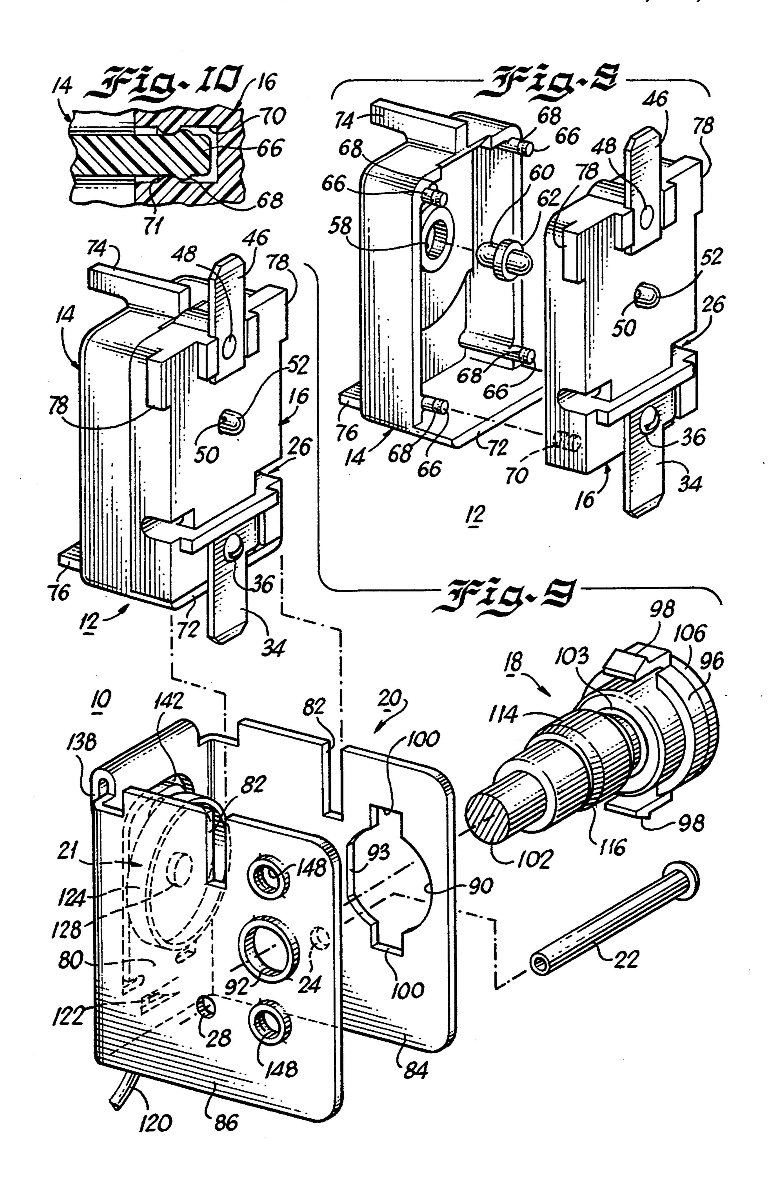
METHOD OF ASSEMBLING A MODULAR ELECTRIC/GAS OVEN THERMOSTAT
