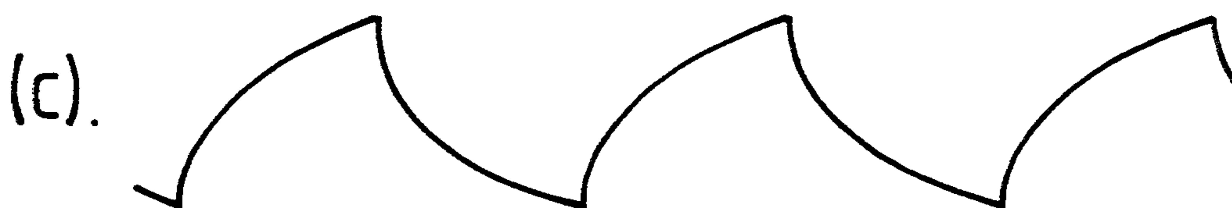
INCREASING CAPACITANCE REDUCES SIGNAL AMPLITUDE
