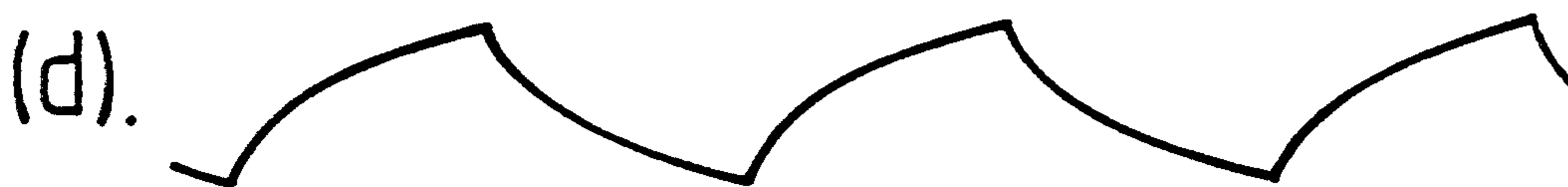
AMPLITUDE DECREASES FURTHER AS CAPACITANCE INCREASES
