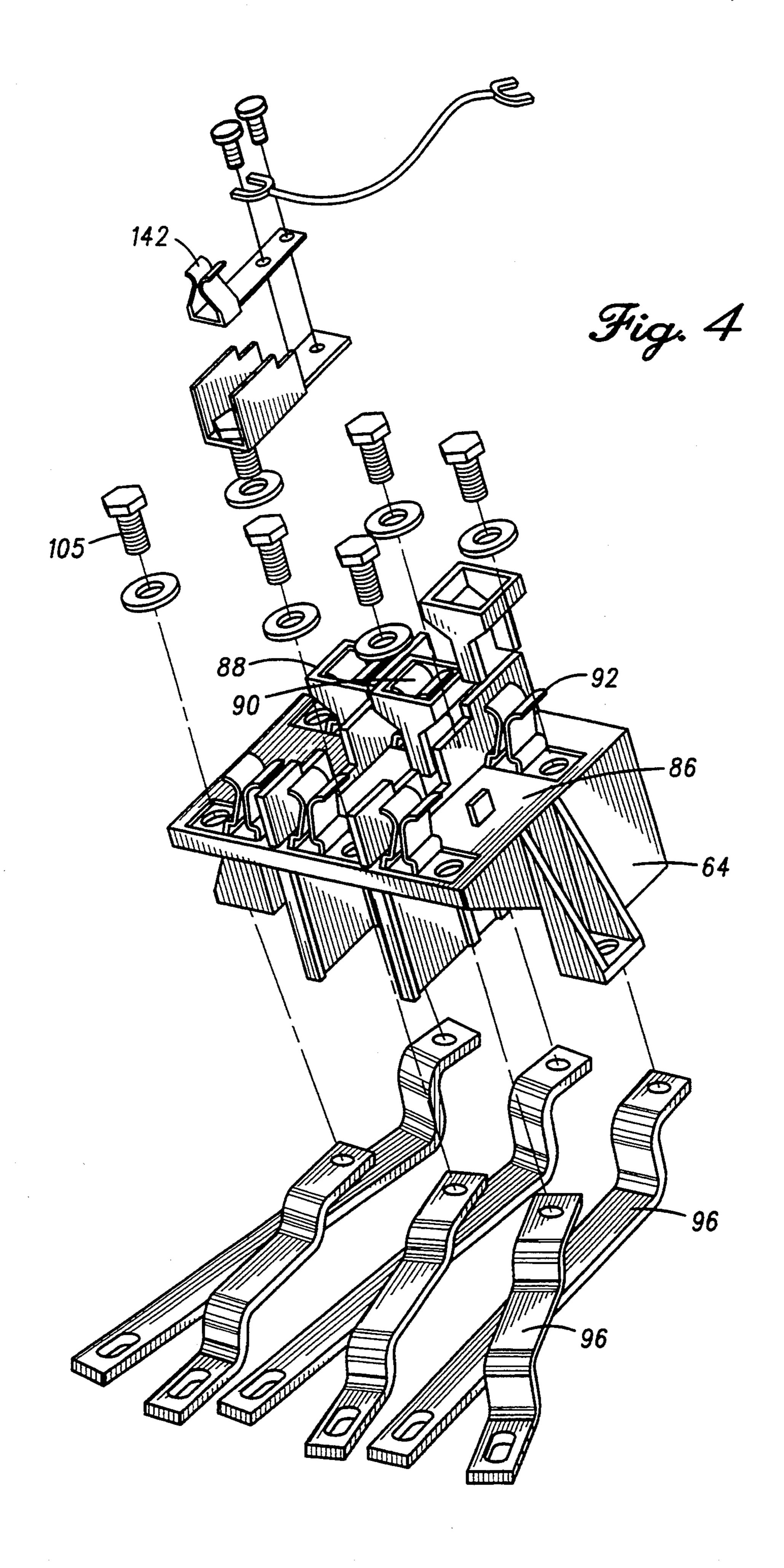
METER SOCKET ASSEMBLY AND DISTRIBUTION BOARD
