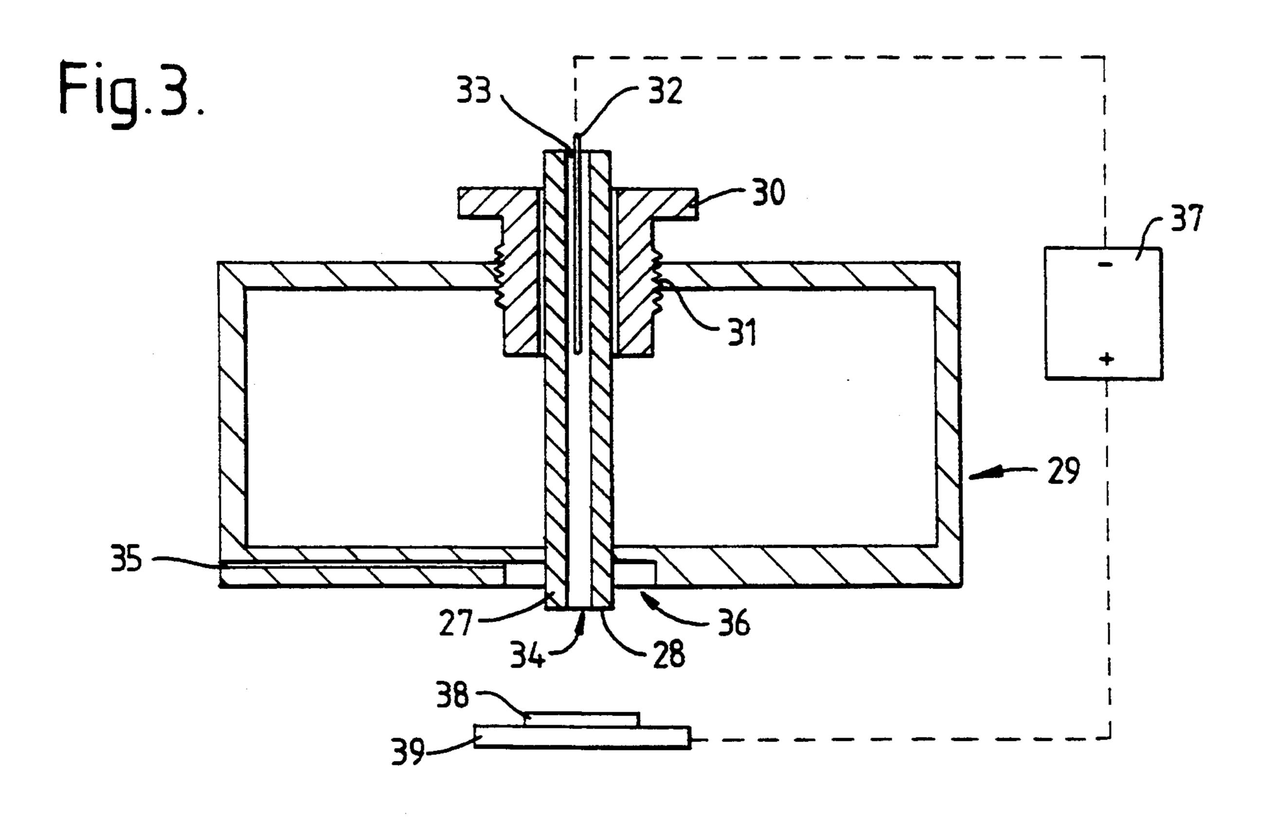
GAS PLASMA GENERATING SYSTEM WITH **RESONANT CAVITY**
