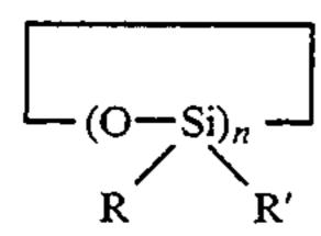
where R is a saturated, substituted or unsubstituted alkyl or alkoxy group or a substituted or unsubstituted aryl or aryloxy group, R' is a substituted or unsubstituted hydrocarbon group having at least one nonaromatic carbon-carbon double bond that is reactive in hydrosilation, and n is 3, or 3 and 4.
