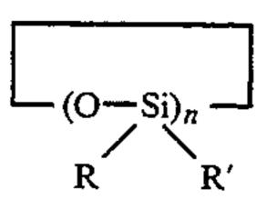
where R and R' are defined below and n=3, or 3 and 4. The notation "3 and 4" means that a mixture of a cyclic trisiloxane (n=3) and a cyclic tetrasiloxane (n=4) is used.
