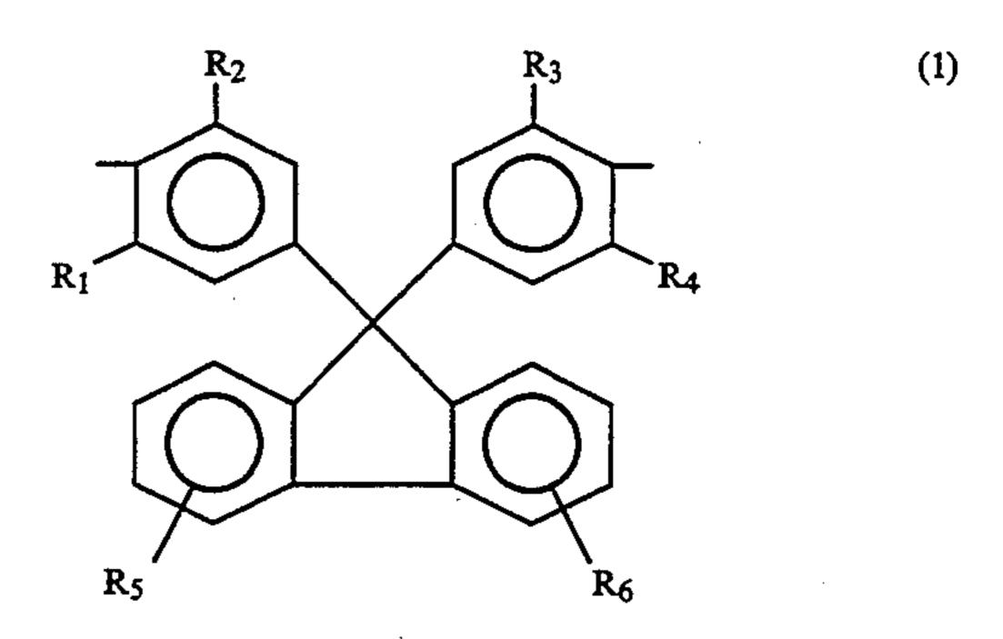
(R<sub>1</sub>, R<sub>2</sub>, R<sub>3</sub>, and R<sub>4</sub> designate hydrogen, alkyl group, and halogen and R<sub>5</sub> and R<sub>6</sub> designate any one of —H, —SO<sub>3</sub>H, —COOH, and —OH) and water or an aqueous solution of substances with affinity for CO<sub>2</sub> substantially uniformly retained in said support membranes.
