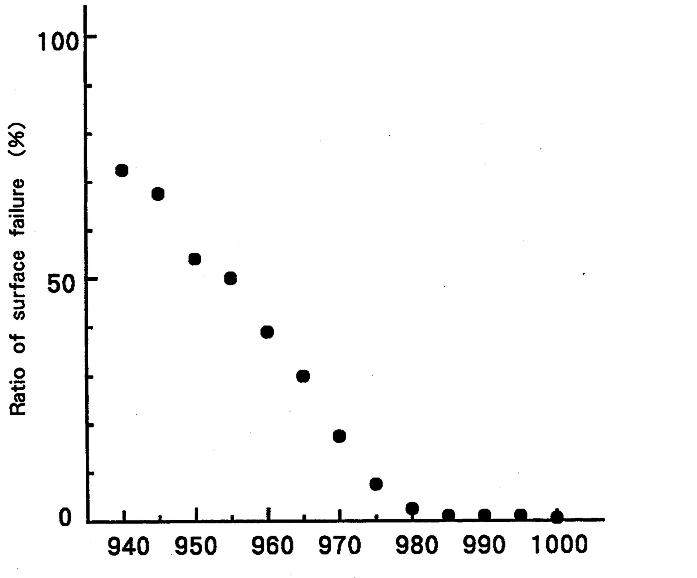
Growth completion temperature T2 of the p-type GaP layer (°C)
