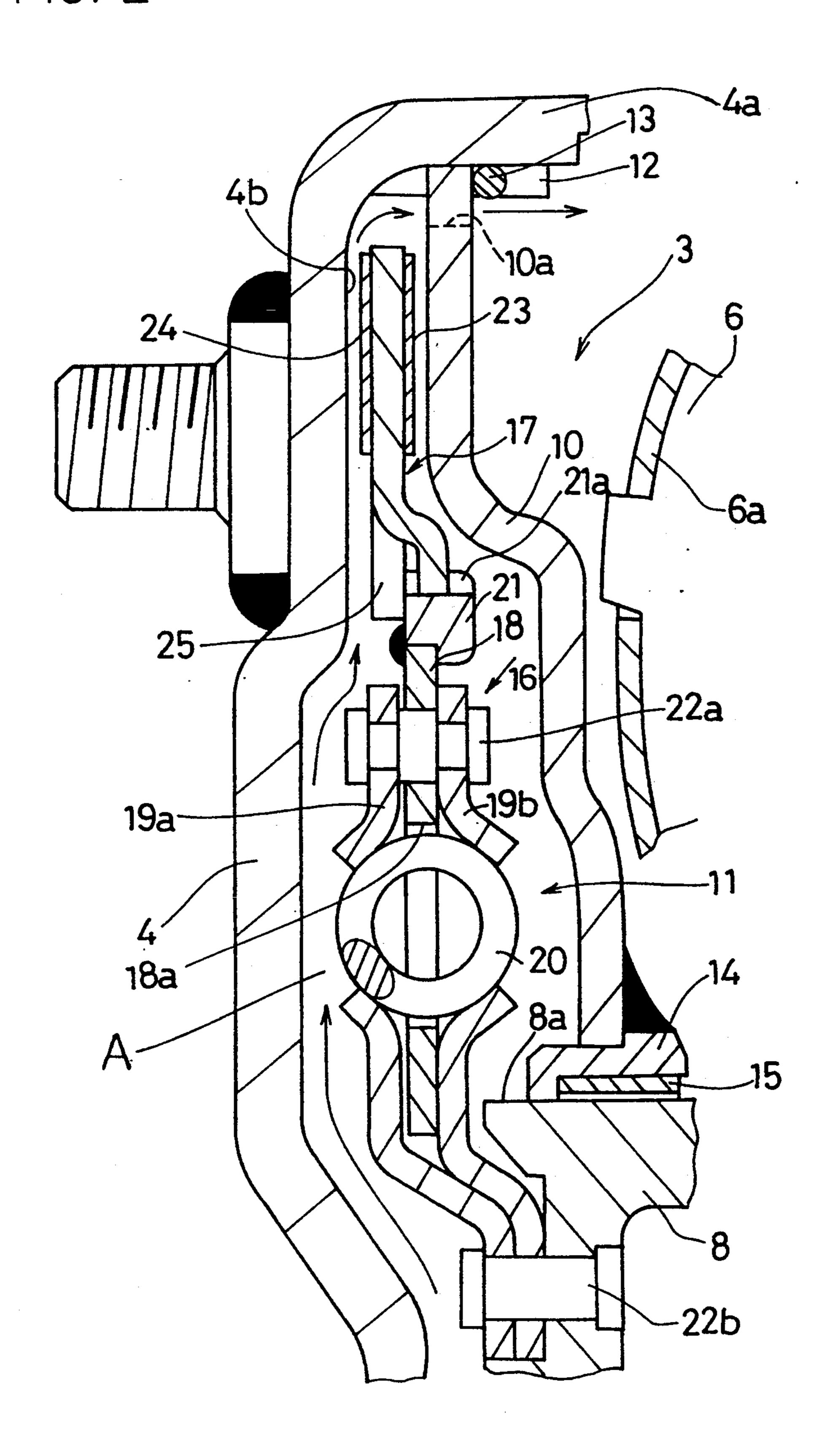
the inner wall of the front cover and the plate member and a frictional surface between the plate member and the piston are frictionally engaged with each other,
