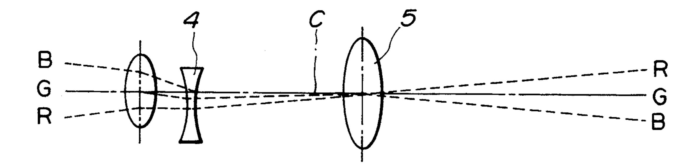
the electron beams are appropriately aligned relative to a central axis.
