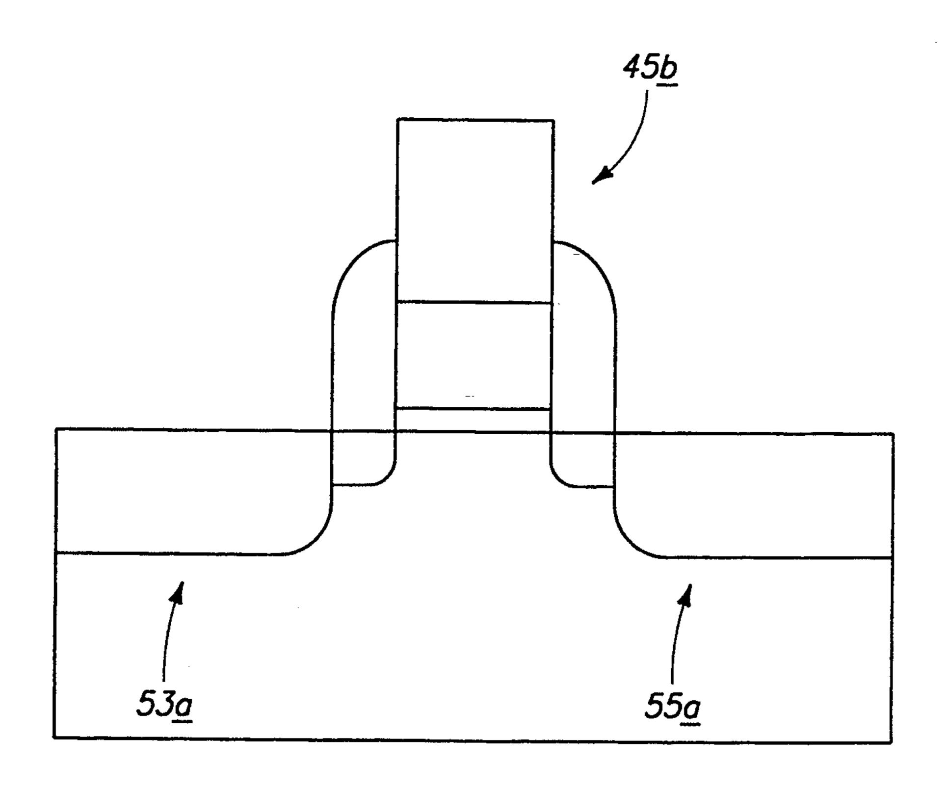
FIG. 1 is a sectional view of a semiconductor wafer fragment at one processing step in accordance with the invention.
