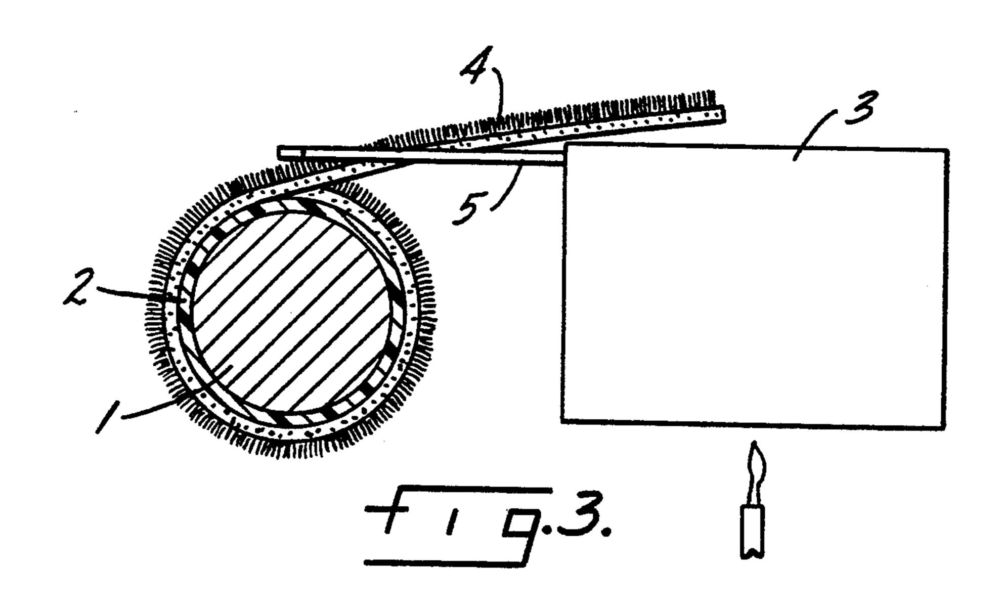
fabric and the plastic tube form a single paint roller
