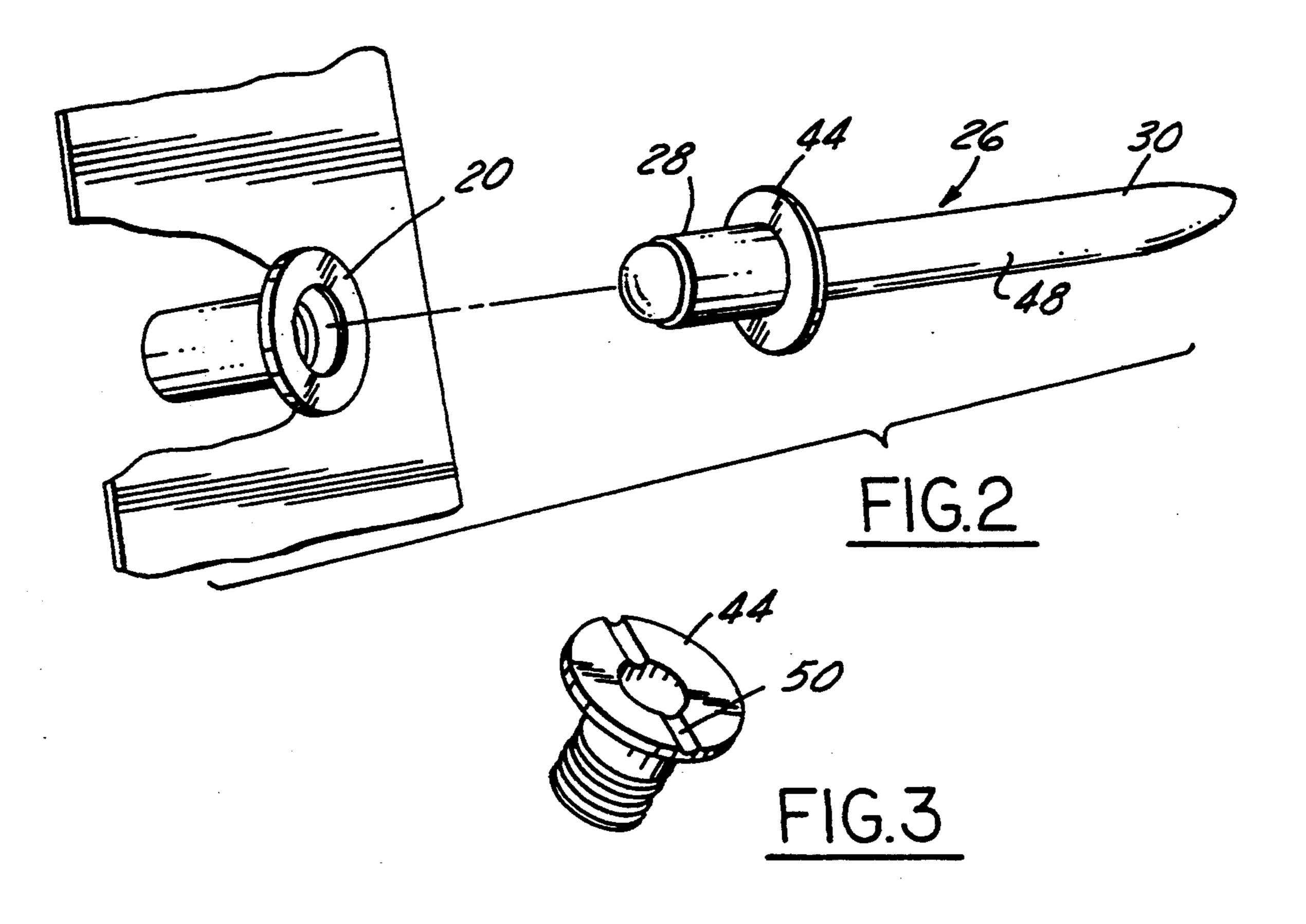
FIG. 3 is a perspective view of the rivet shell of the fastener of the present invention in its formed condition.
