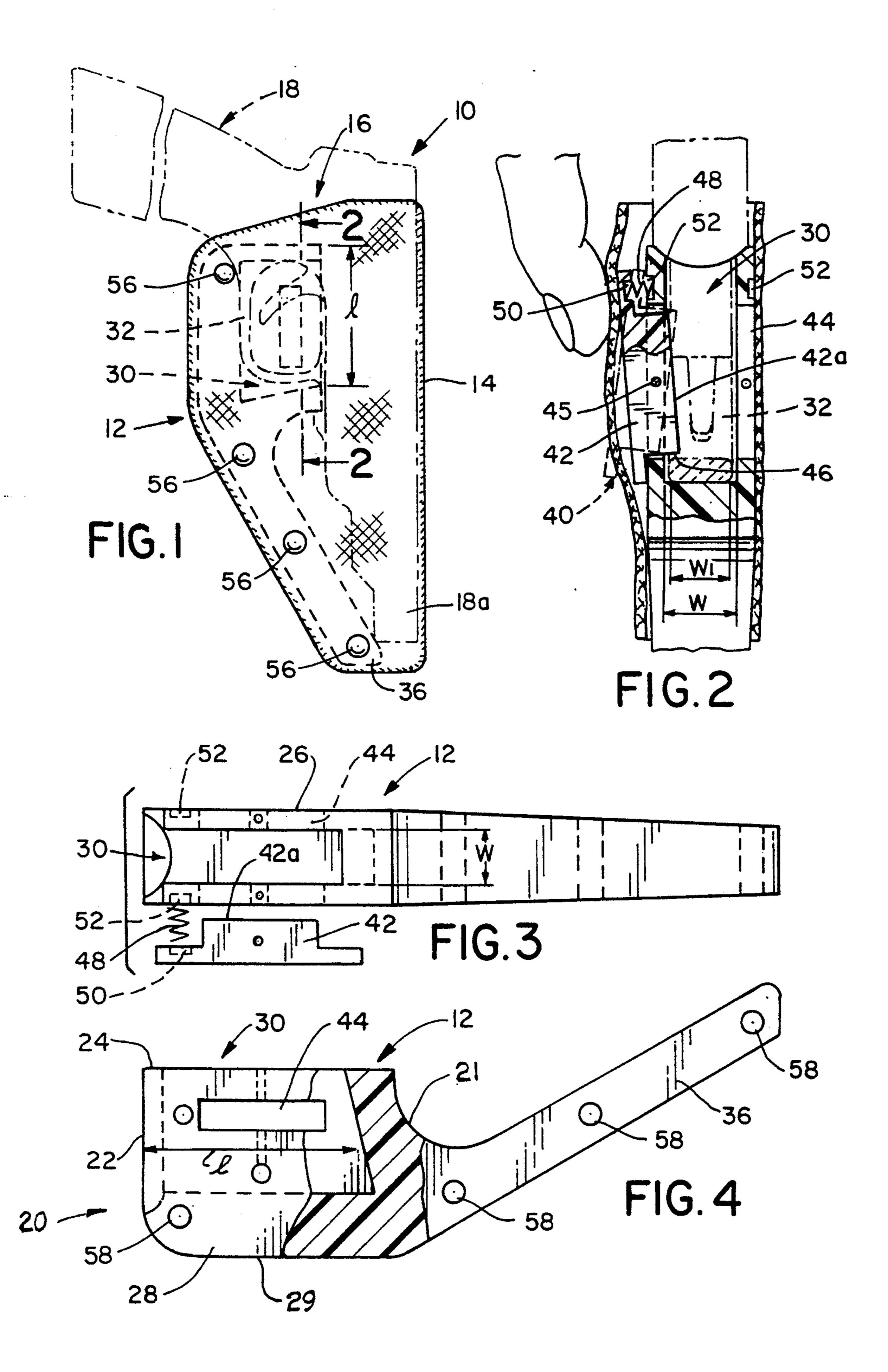
unitary, one-piece structure. Also, the latch is preferably positioned in the main body for pivotal movement about an axis that is located laterally of, and generally parallel to, the slot.
