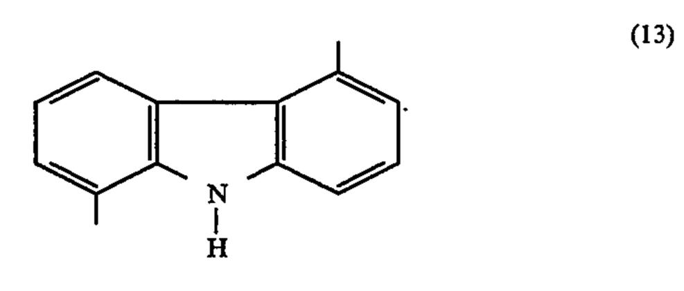
21. The insulated wire according to claim 7, wherein said at least one resin comprises a repeating unit of the formula:
