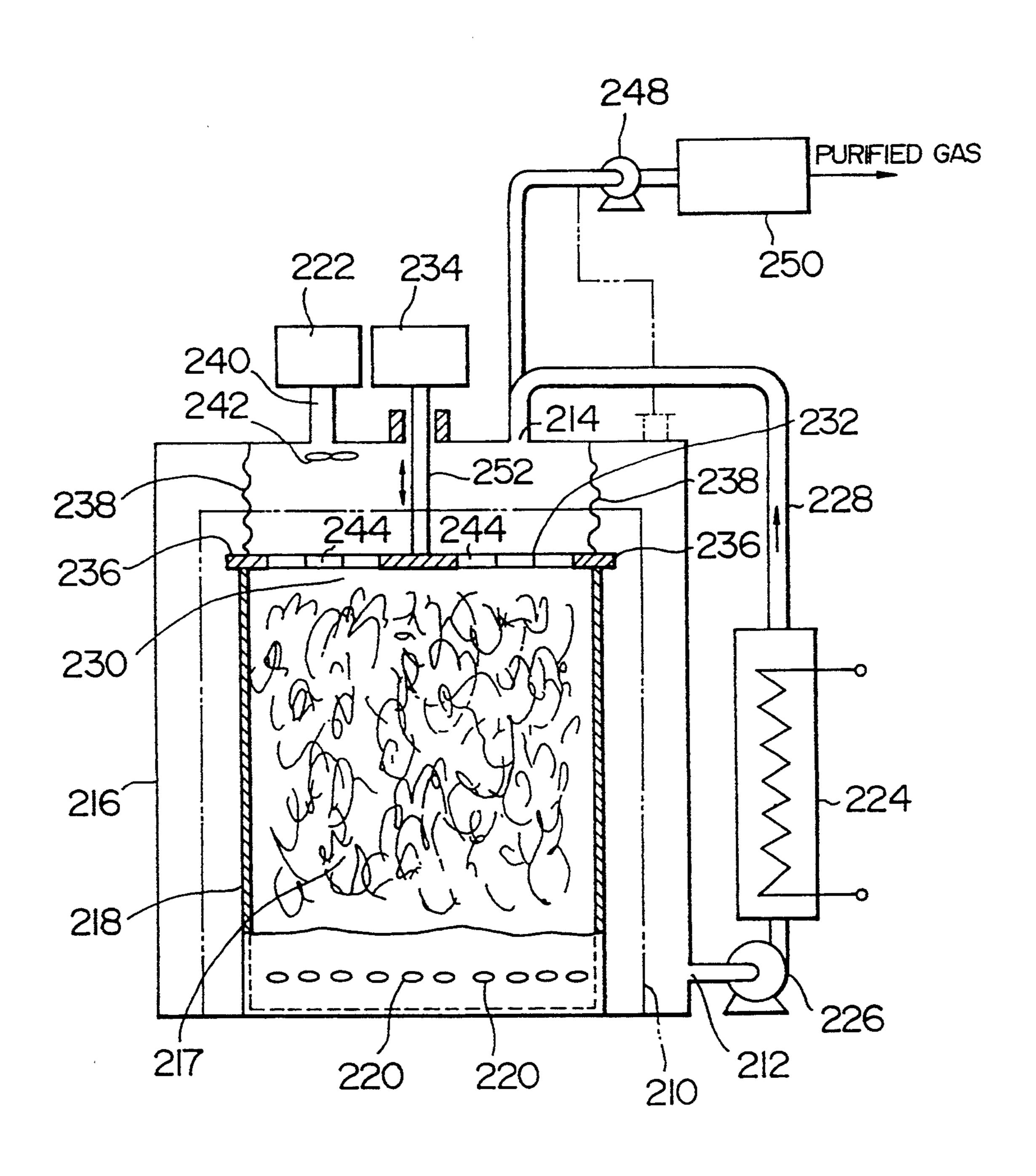
APPARATUS FOR TREATING INFECTIOUS MEDICAL WASTES WITH MICROWAVES AND HOT AIR
