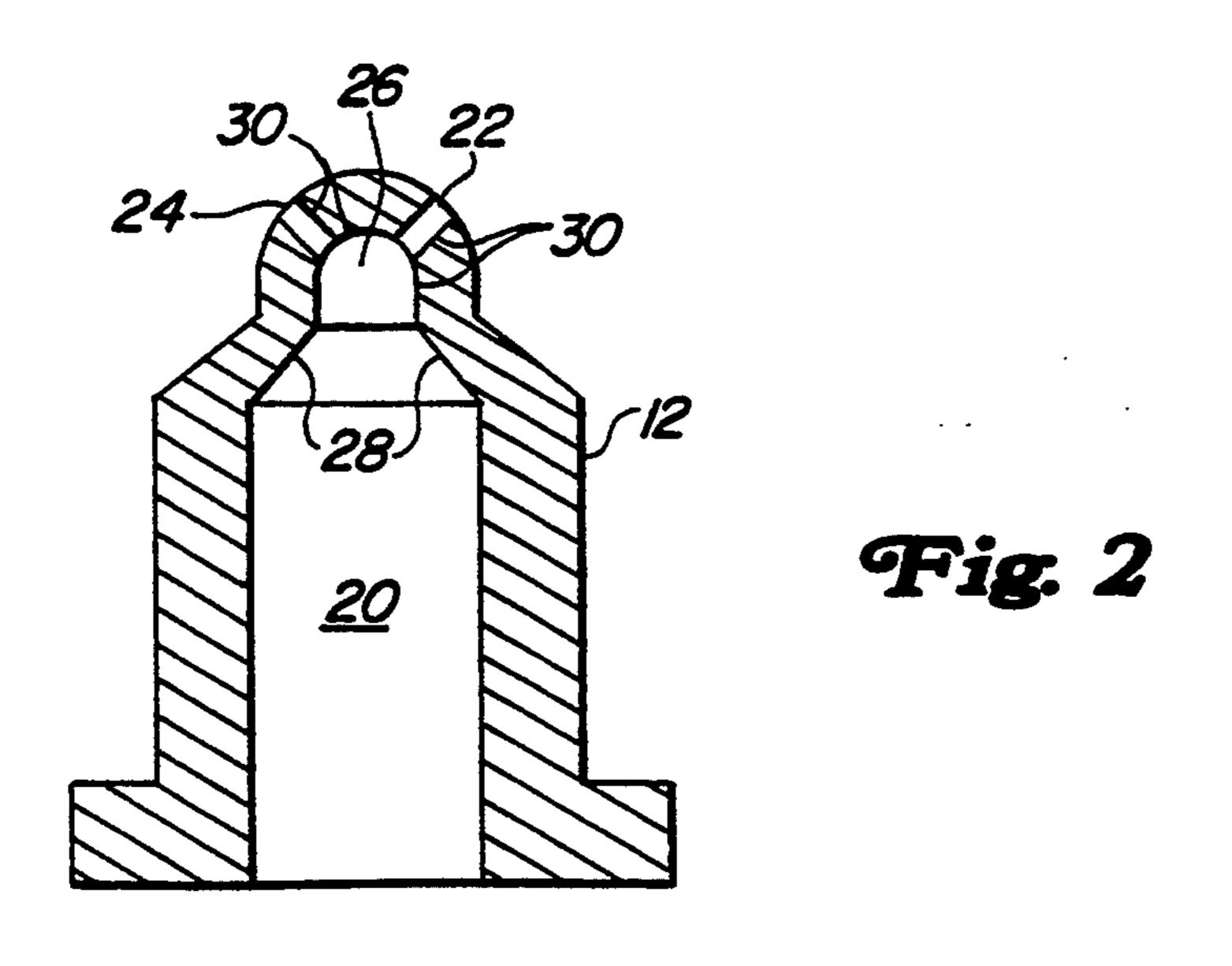
APPARATUS FOR DEPOSITING HARD COATING IN A NOZZLE ORIFICE
