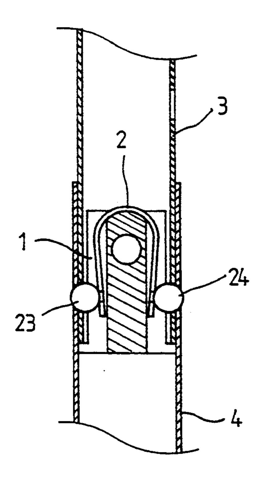
SECURING MEANS FOR TELESCOPIC STICKS OF A MULTIPLE-FOLD UMBRELLA
