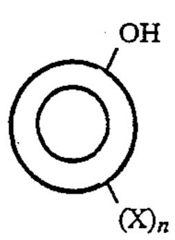
wherein  $\odot$  is a 5- or 6-membered, heterocyclic or nonheterocyclic, monocyclic or multicyclic aromatic ring; X is an electron-withdrawing group; and n is 0, 1, 2 or 3 with the proviso that (1) n cannot be zero when the aromatic ring is benzene and (2) the locations of OH and X on the aromatic ring are such that the overall compound has a pKa within the range from about 5 to 9.7.
