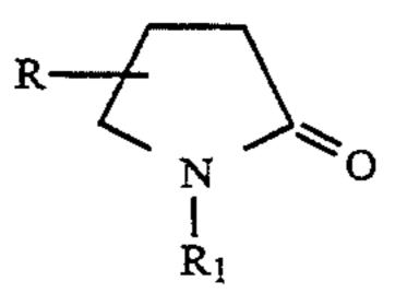
where R is hydrogen or lower alkyl and R<sub>1</sub> is lower alkyl, cyclic lactones, lower alkyl cyclic carbonates, lower alkyl imidazolone, lower alkylamides of formic and acetic acid, and lower alkyl sulfoxides, wherein lower alkyl is an alkyl group having from 1 to 4 carbon atoms.
